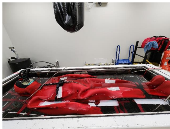
Figure 3: TIM secured on the stretcher in the TML immersion tank.
