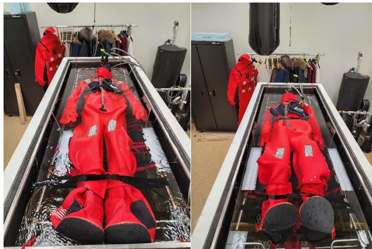
Figure 10: TIM (left) and NEMO (right) in the Survivtec immersion ensemble in the immersion tank.
