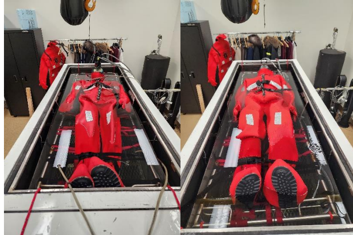
Figure 9: TIM (left) and NEMO (right) in the Mullion immersion ensemble in the immersion tank.
