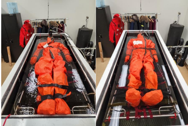
Figure 11: TIM (left) and NEMO (right) in the Viking immersion ensemble in the immersion tank.
