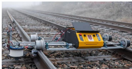
Figure 4. Image of a prototype mobile robot for installing fibre optic sensors on railways
