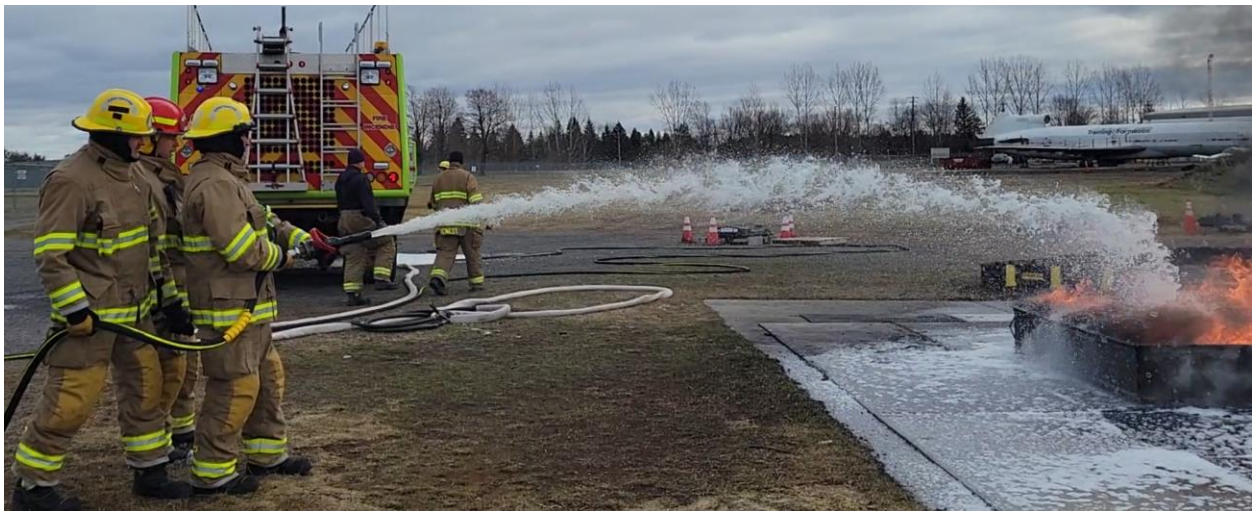
Figure 2 Handheld application using a firehose as per OIAA practices with the OIAA CAF system
