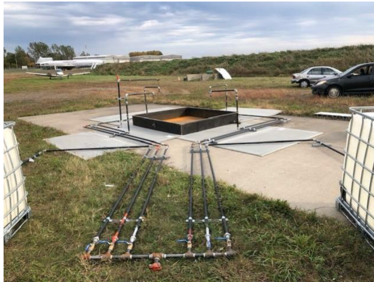
Figure 1 Fireflex ICAF system for the topside application
