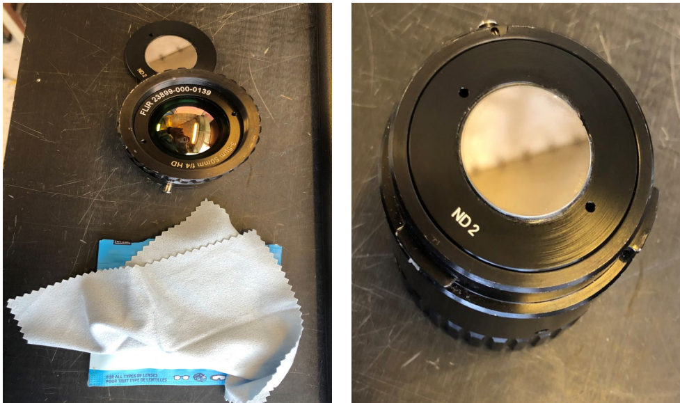
Figure 13 – ND2 filter cleaned and attached on the back of lens before calibration.
