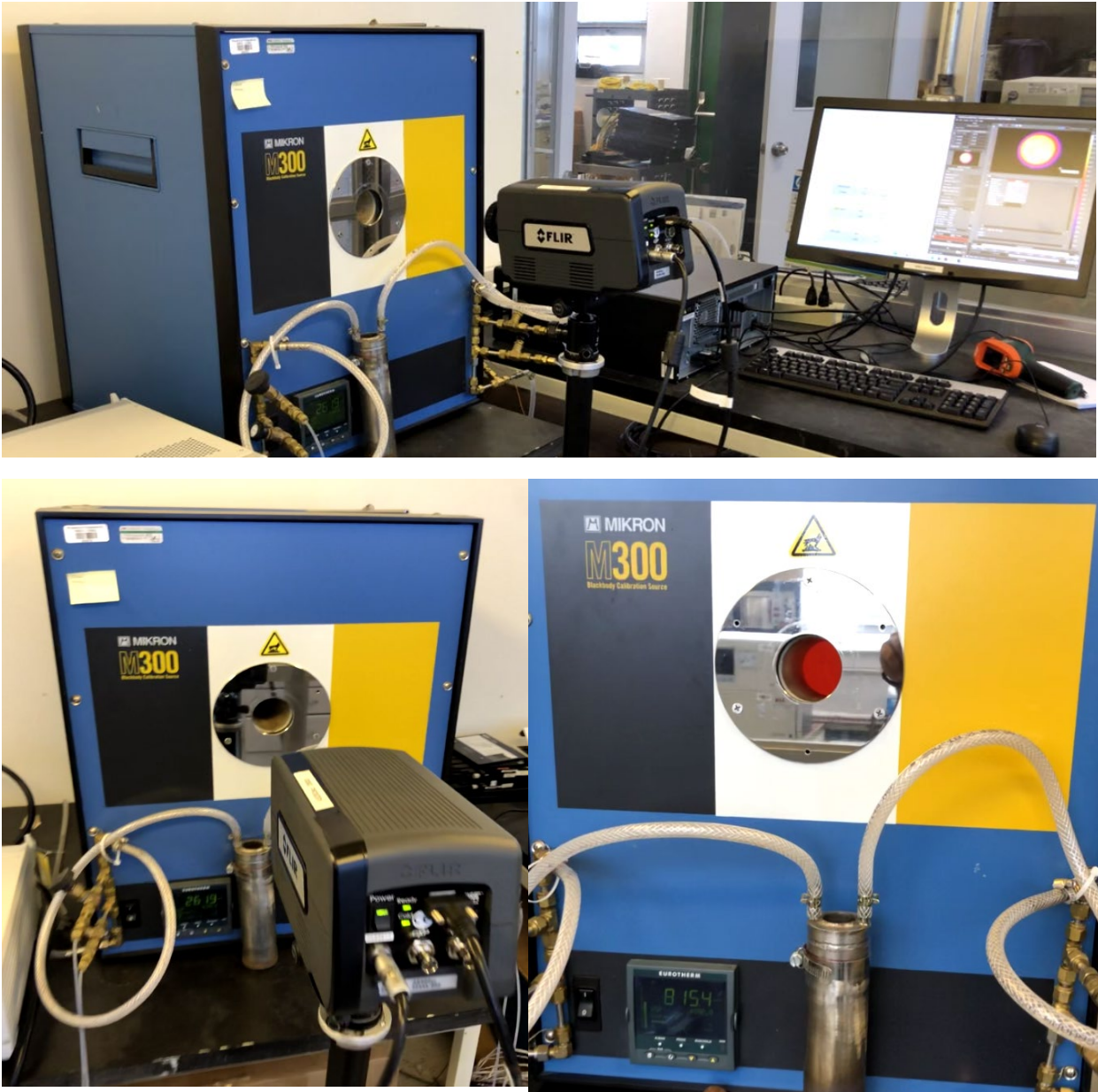
Figure 10 - Different angles of Cavity blackbody use in the calibration process when FLIR A8303sc pointed to the cavity with temperature around 800°C.
