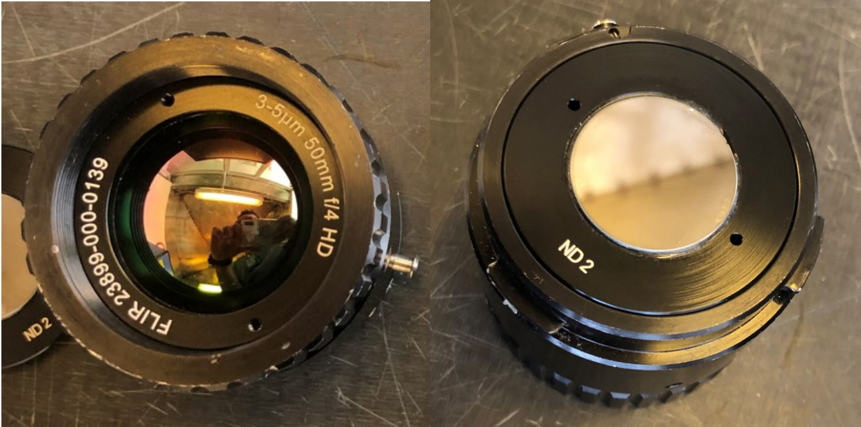
Figure 8 - FLIR 50mm f/4 HD lens for using with MWIR camera. On the right, ND2 filter attached on the back of Camera Lens.
