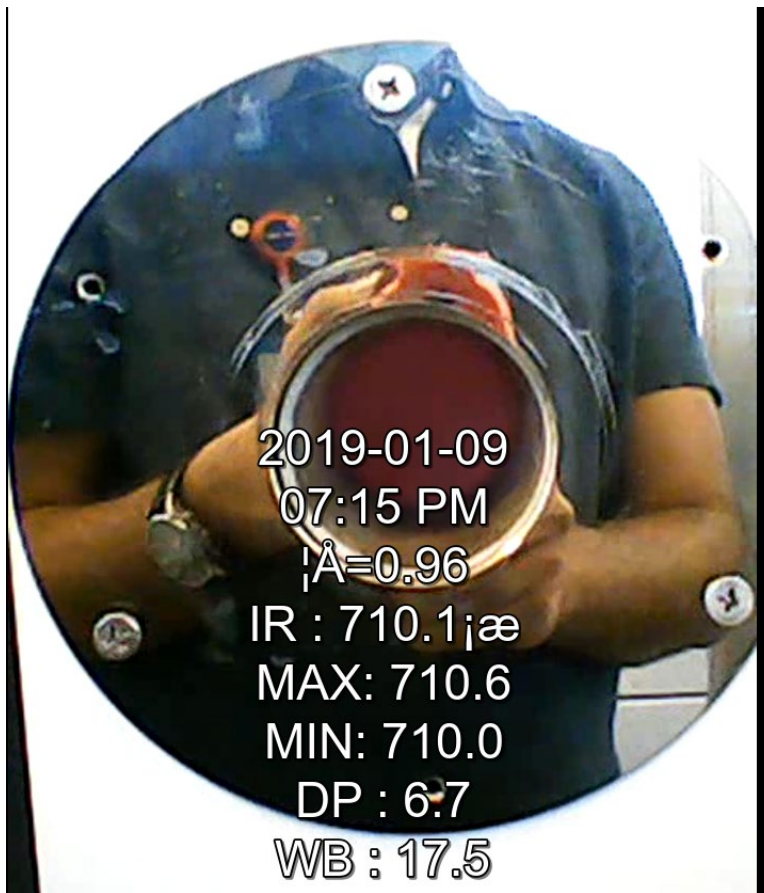
Figure 26 – IR thermometer temperature reading of blackbody with cavity set on 700°C
