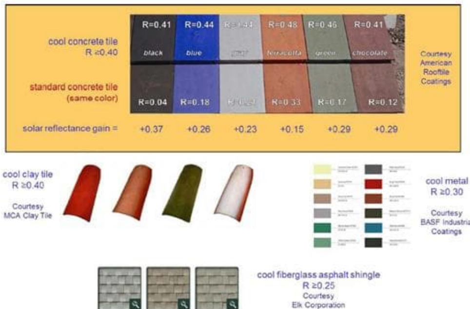
Figure 7: Examples of cool-colored roofing materials in the market. R is solar reflectance. Image created by (author/NRC), informed by: Heat Island Group, Lawrence Berkeley National Laboratory, Berkeley, California, USA. (U.S. DOE, 2010)
