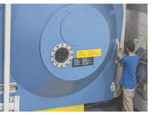
The NRC's altitude research facility makes it possible to evaluate engines and components under simulated conditions and burning different fuels.
