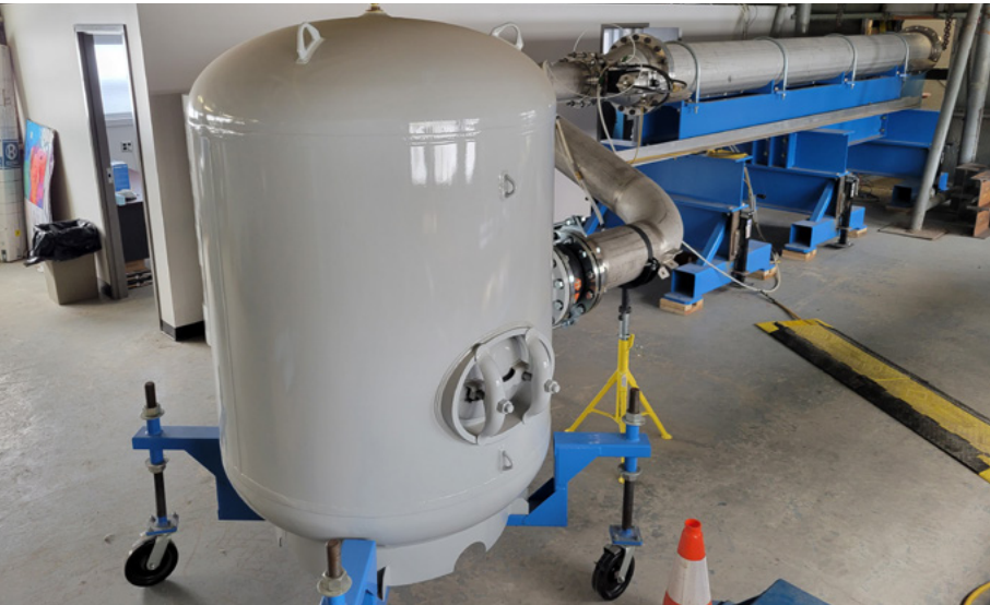
The NRC's drone super cannon is used for drone impact testing and research.
