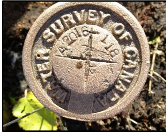
Figure 2: An image of a WSC benchmark complete with a benchmark identifier.
