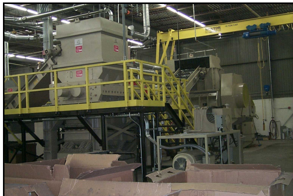
Photo 1. An industrial scale e-waste shredding machine
