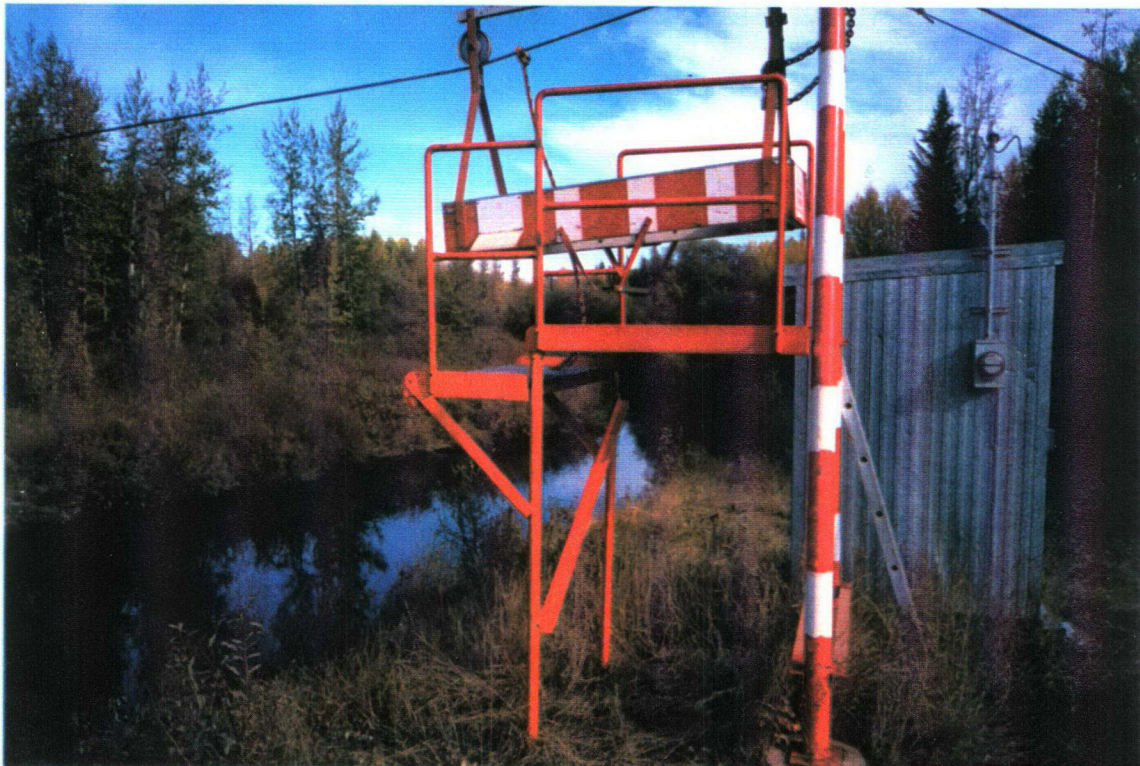
TYPICAL SITE SHOWING CABLEWAY TOWER AND INSTRUMENT SHELTER JACKPINE CREEK AT WADLIN LAKE ROAD 21-SEPTEMBER-95
