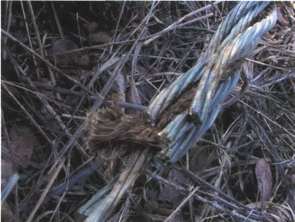
Figure 6: Notikewin River/Manning, Vandalized LB main cable, Apr 2005
