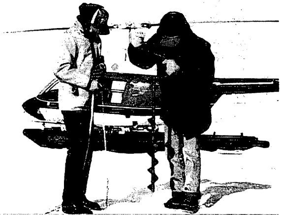
Measuring ice thickness on Lake Erie.
