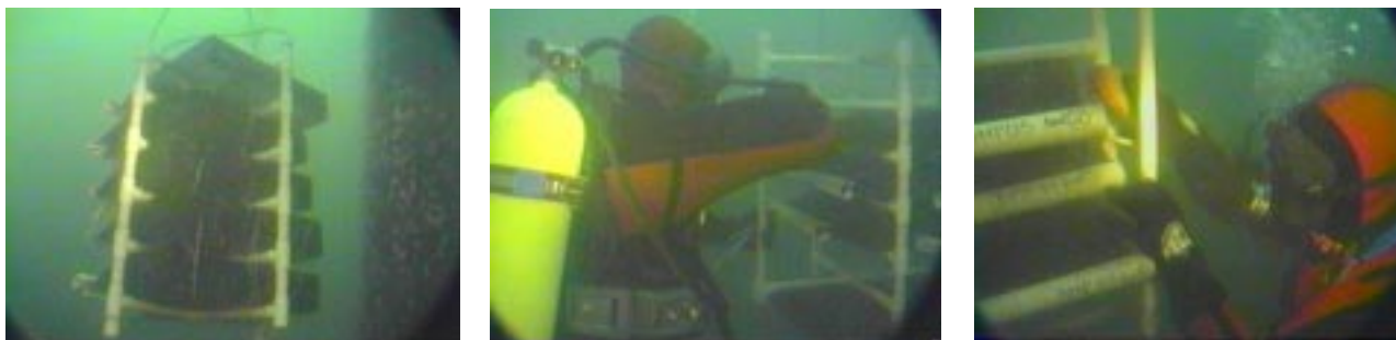
Figure 8. Photographs of cages used to house mussels ( Mytilus edulis edulis ) for in-situ bioassay during the 1995-1996 Sooke Basin Creosote Evaluation Study.
