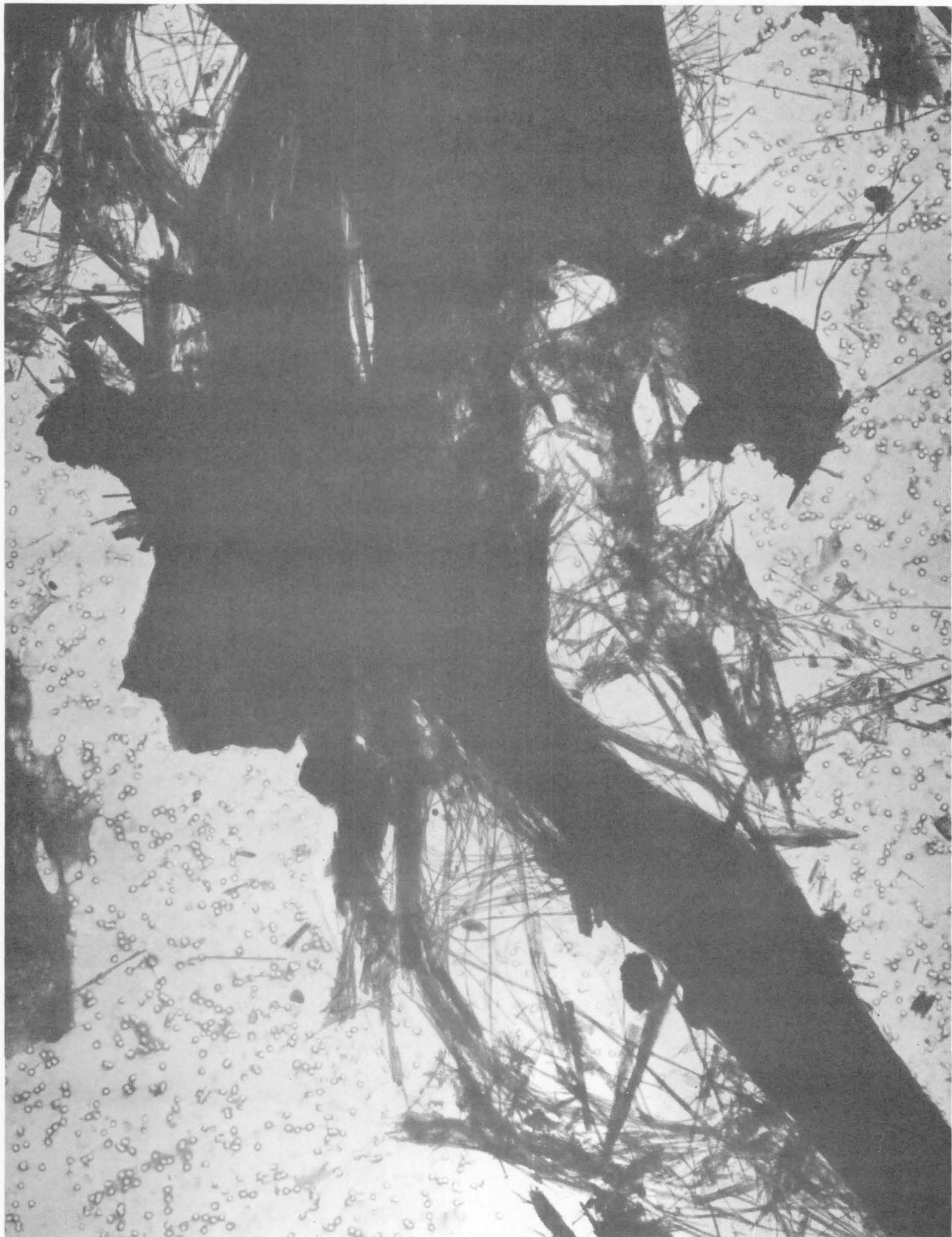
FIGURE 8 - Indirect method - Chrysotile bundle persisting after ultrasound treatment for 7 minutes
