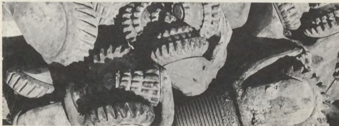
More than 100 of these rotary bits are required to drill a single well.
