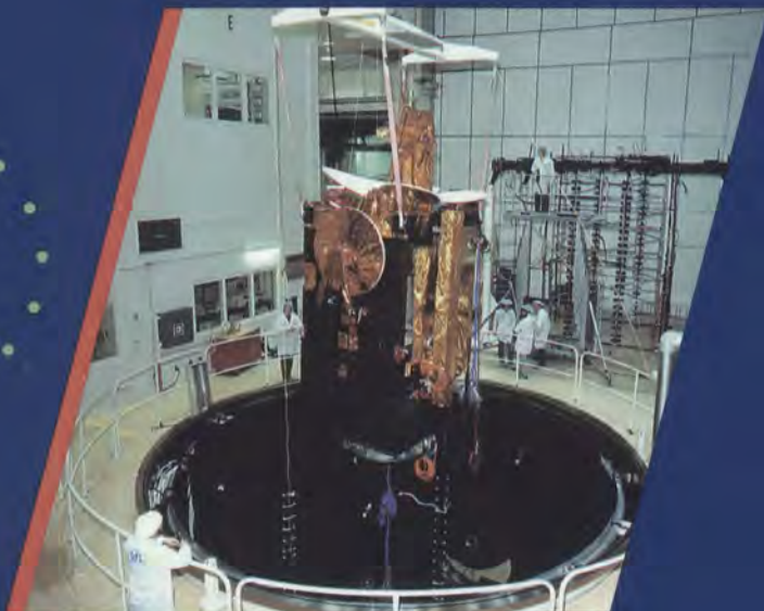
European Space Agency's Olympus Satellite Thermal Model, Thermal Vacuum Appendage Release Test
