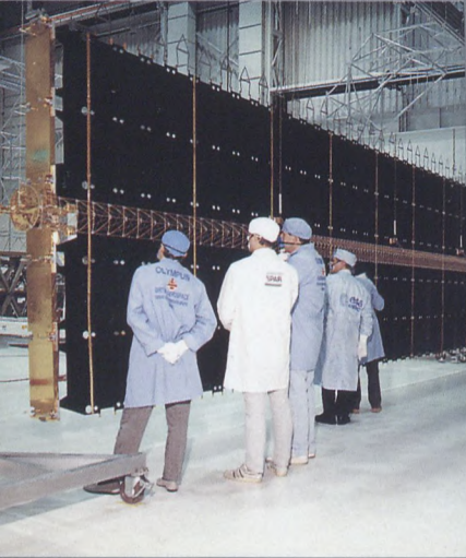
■ Solar array deployment at the David Florida Laboratory.
