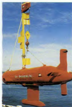
DOLPHIN, a remotely operated vehicle (ROV), maps the ocean floor. Courtesy of Geo-Resources Inc.
