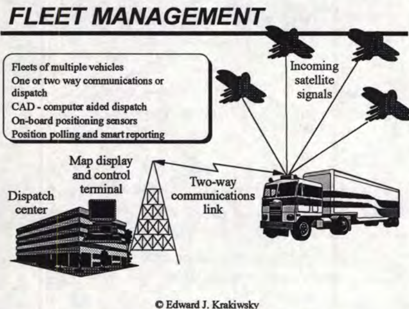
Figure 23-1: A Generic Fleet Management IVHS Navigation System
