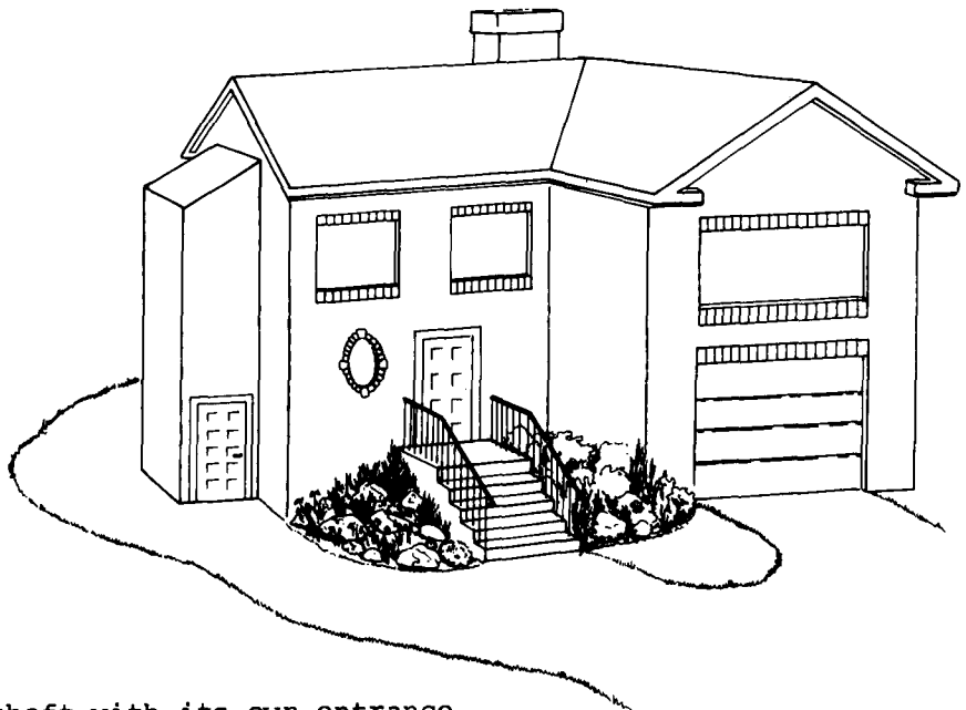
An exterior elevator shaft with its own entrance
