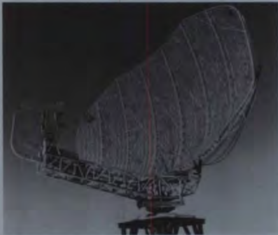
S-band surveillance radar antenna constructed by Andrew for India.
