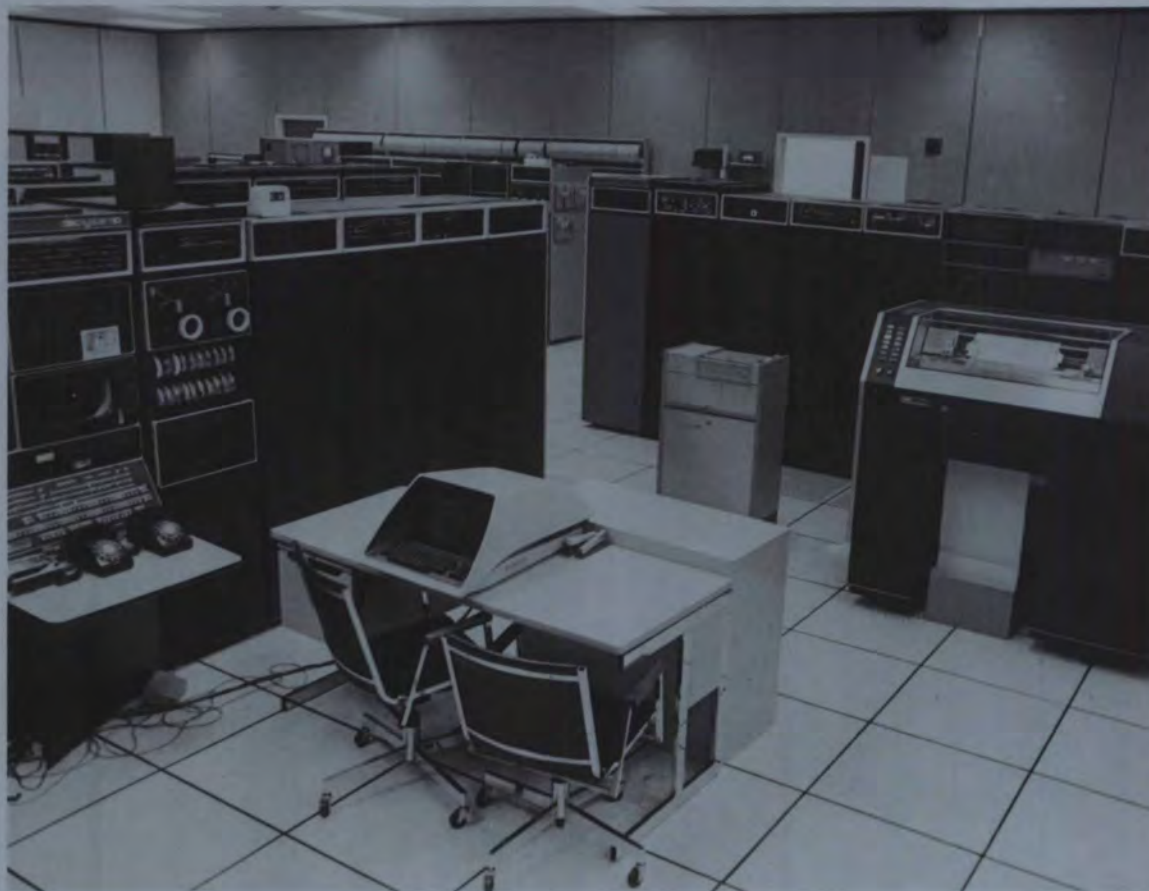
The PDP-10 time-sharing computer system in CCRS laboratories is used to preprocess LANDSAT data, to process digital airborne data and to digitally analyse and enhance MSS data.
