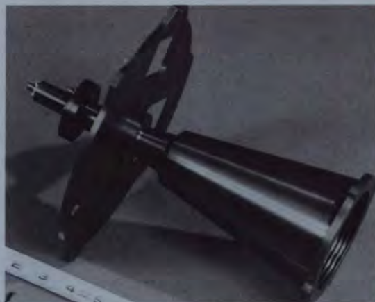
Monopulse antenna used with the microwave attitude sensing system for the Japanese Broadcast Satellite.
