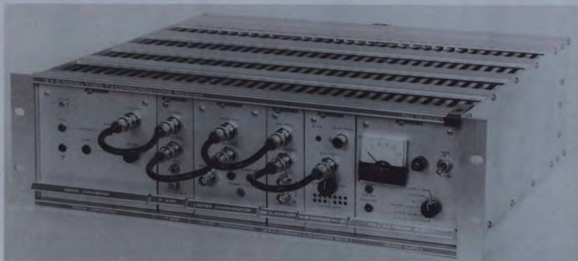
Satellite communications television receiver. Designed and fabricated by SED Systems Ltd. for Telesat Canada, it operates in the 3.7 to 4.2 GHz band.
