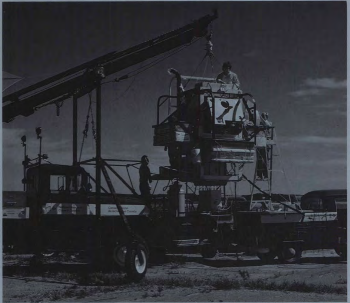
Balloon payload being readied at NRCC mobile balloon launch facility, designed and built by SED Systems Ltd.
