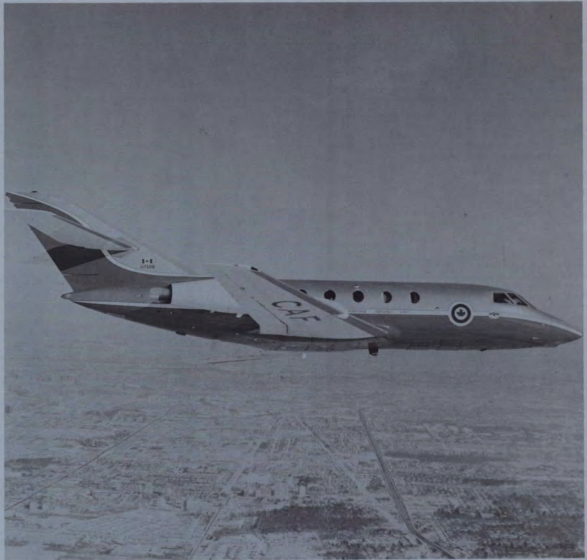
The Dassault Falcon Fan Jet provides CCRS with a high-altitude airborne sensor platform with the ability to reach distant areas quickly.
