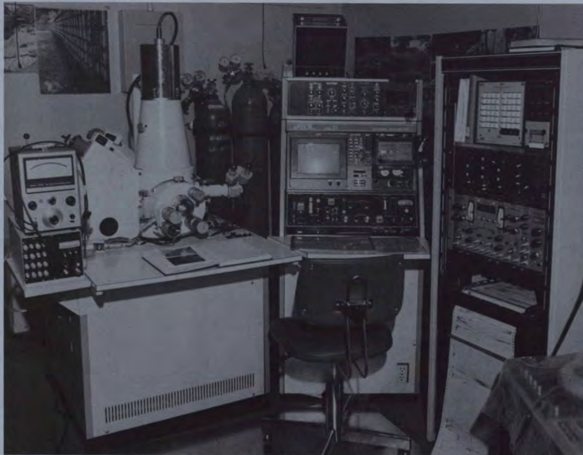
Scanning electron microscope with integral microprobe analyser used for reliability assessment and failure analysis of electronic materials and devices at the Communications Research Centre.
