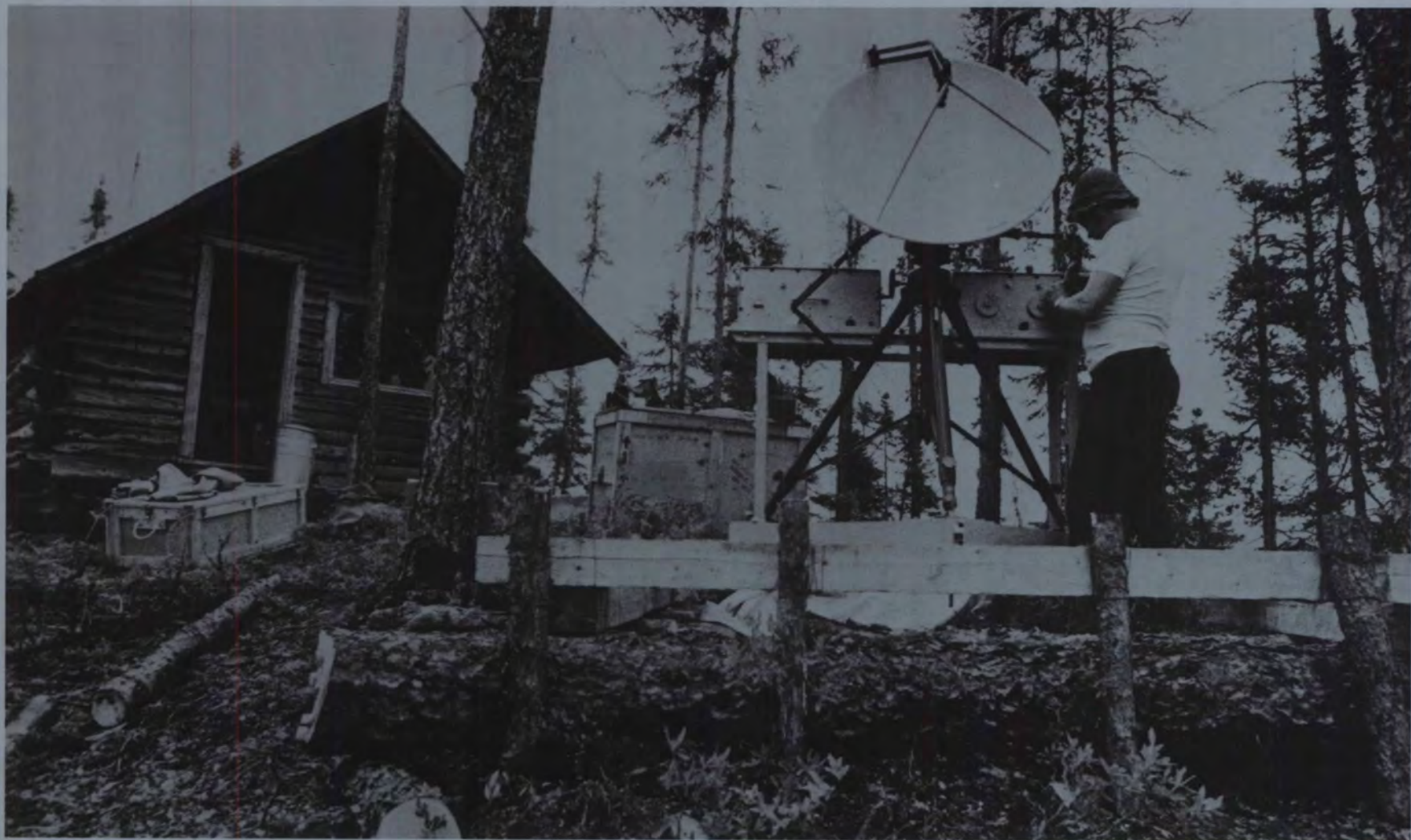
This low-cost ground terminal for voice communication was transported to the site by Otter aircraft and canoe. This photograph was taken during a geological experiment in the James Bay area of Québec.
