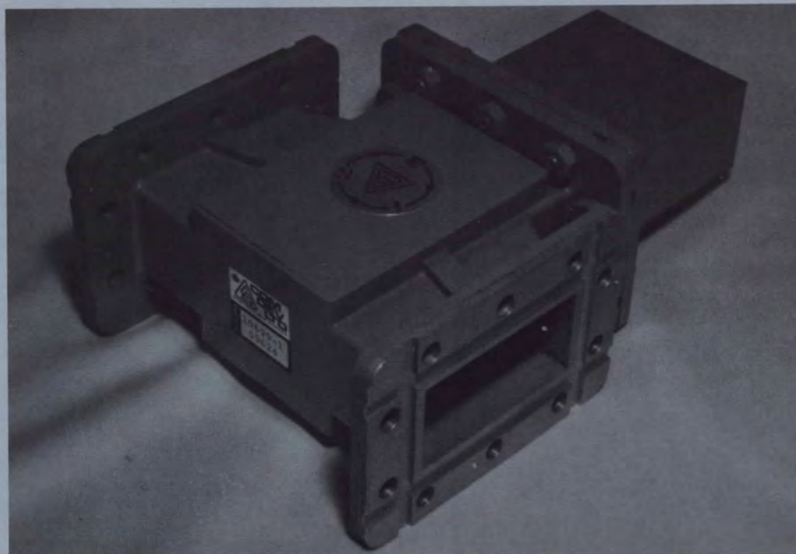
Ferrite technology Waveguide circulator
