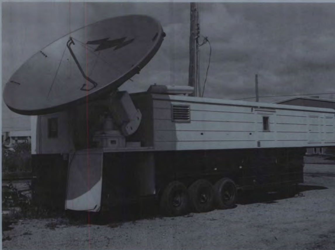
Mobile earth station designed and built by SED for the HERMES satellite.
