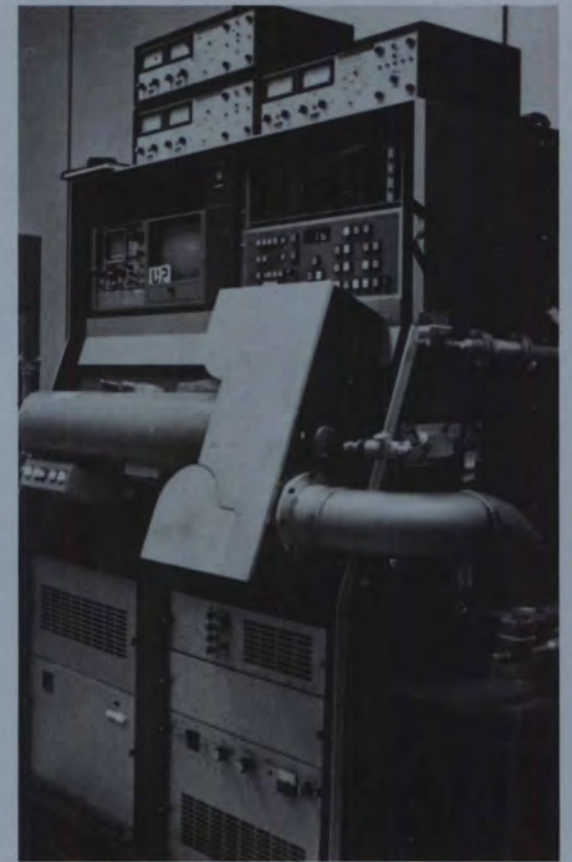
All the high resolution imagery from the LANDSAT spacecraft produced by CCRS has been done on these electron beam image recorders. Electrons write the images on 70mm film in these machines.
