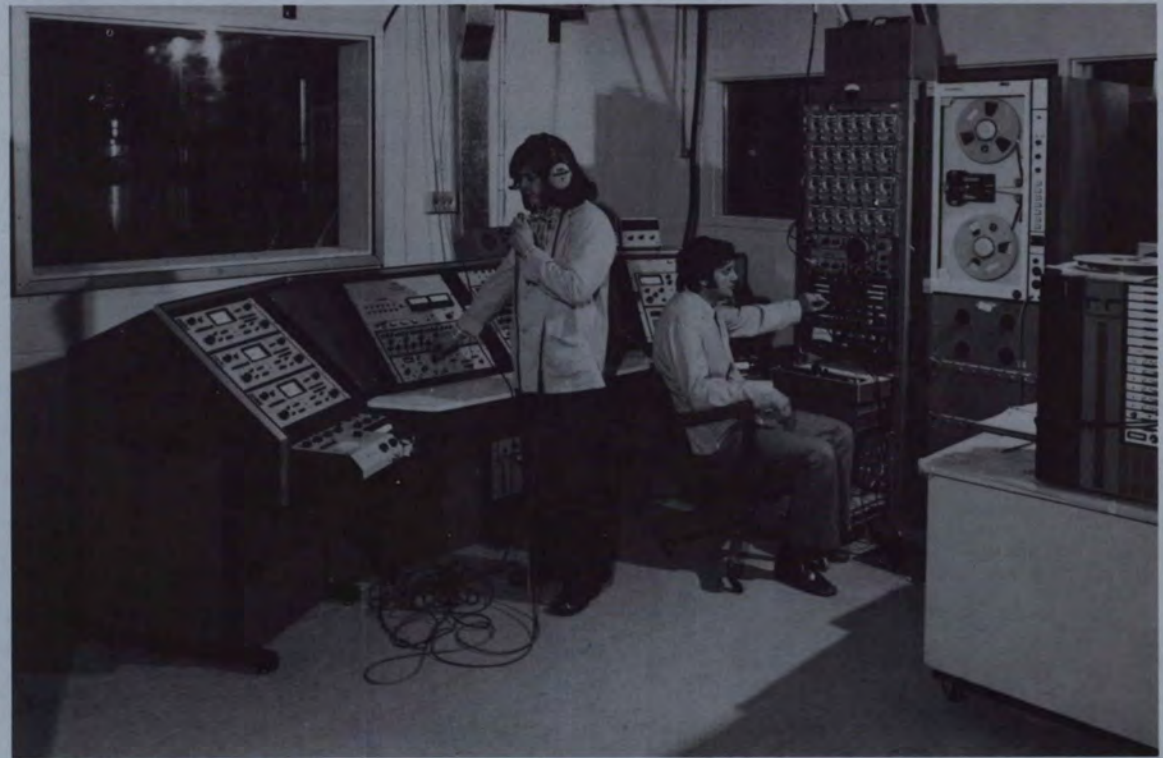
DFL Vibration Facility Control Room. Acceleration and strain can be monitored at up to 42 points simultaneously. The console can also be preprogrammed to simulate tests and a safety system automatically shuts off vibration if the acceleration exceeds programmed test limits.
