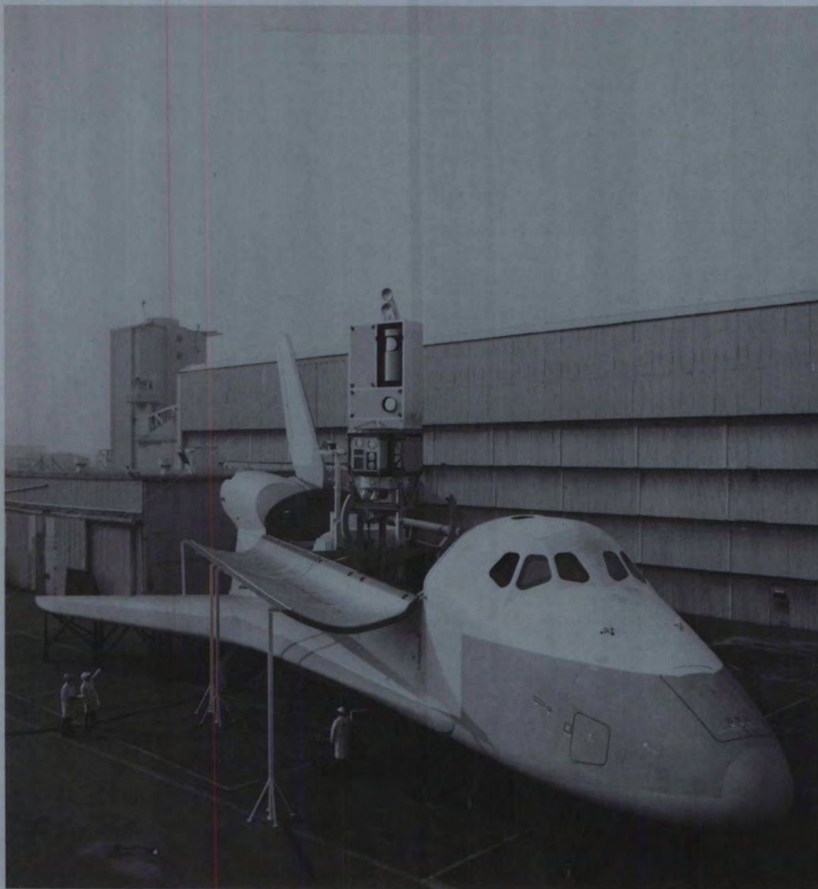
Full-scale mock-up of the Space Shuttle Orbiter with modular exchange mechanism and, behind it, the Remote Manipulator System arm, seen at Rockwell International's facility at Downey, Calif.
