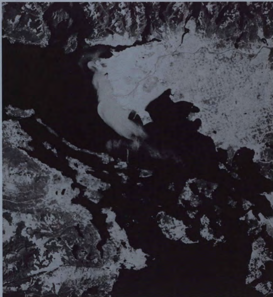
LANDSAT image over Vancouver/Victoria area. The plume of fresh muddy water as it flows out from the mouth of the Fraser River into the clearer salt water of the Strait of Georgia can be seen.
