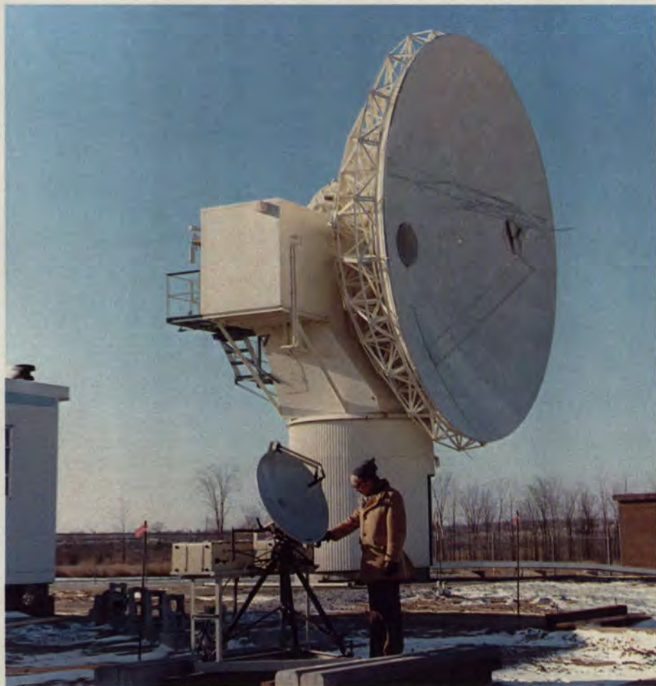
A check-out on one of the 81 cm. diameter earth stations used in direct-to-home communications field trials
