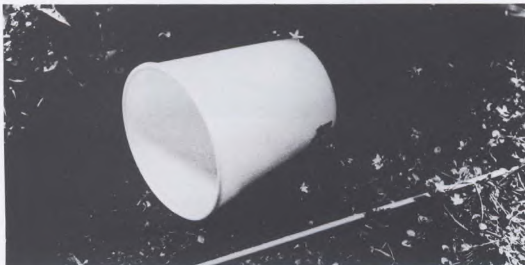
A cup made of Ecolyte Polystyrene and "straw" made of ordinary plastic before exposure to sunlight.
