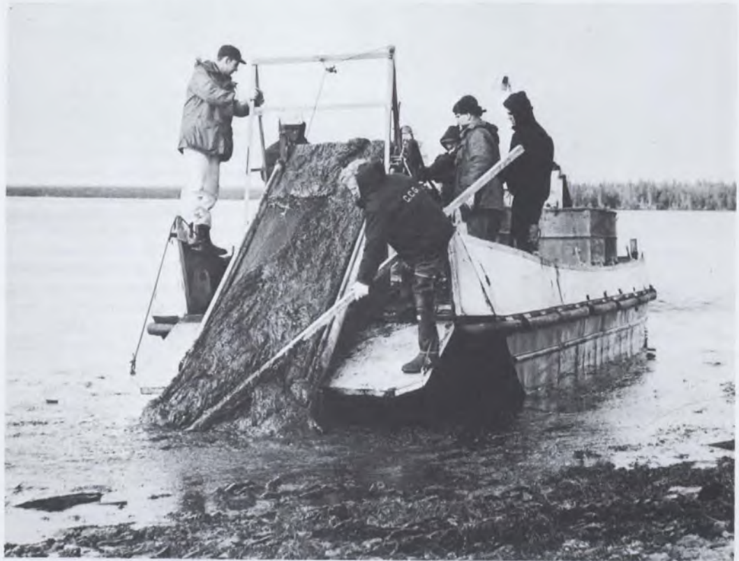
The slicklicker in action in 1970 cleaning up the major oil spill caused by the tanker Arrow in Chedabucto Bay, Nova Scotia.
