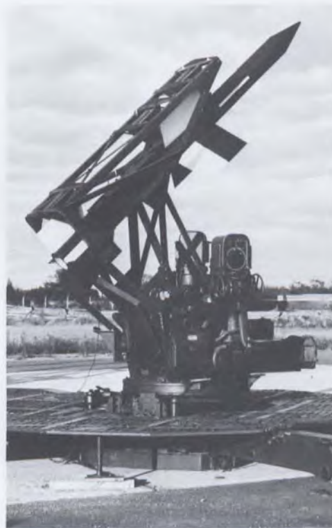
A later version of the Velvet Glove, with its own booster, is ready for a flight trial at the Defence Research Board's Picton Range late in 1954.
