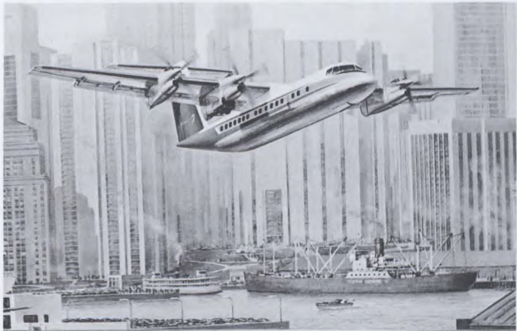
The DHC-7 'Quiet STOL Airliner' designed by de Havilland Canada for short hauls.
