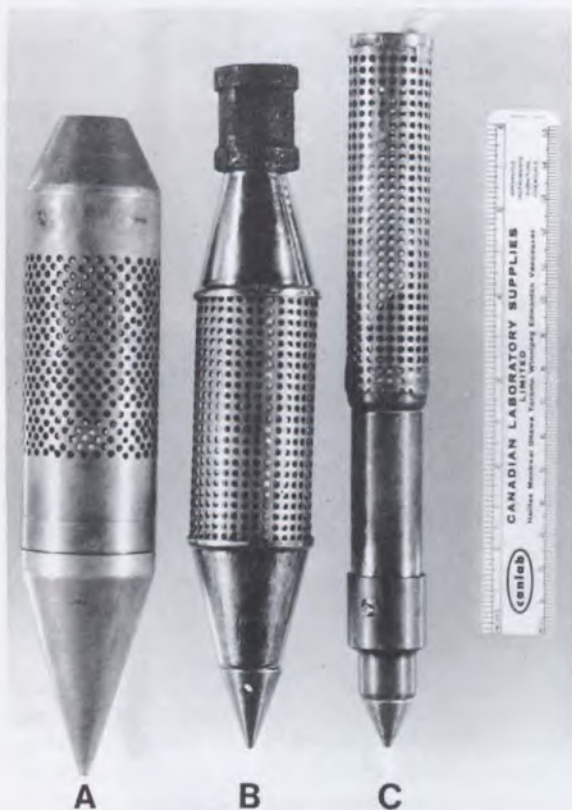
These are three versions of grain insect detection devices. (A) is the earliest model, made in 1967. (B) is an economical version, produced in 1969. (C) is the latest improved model of 1973.
