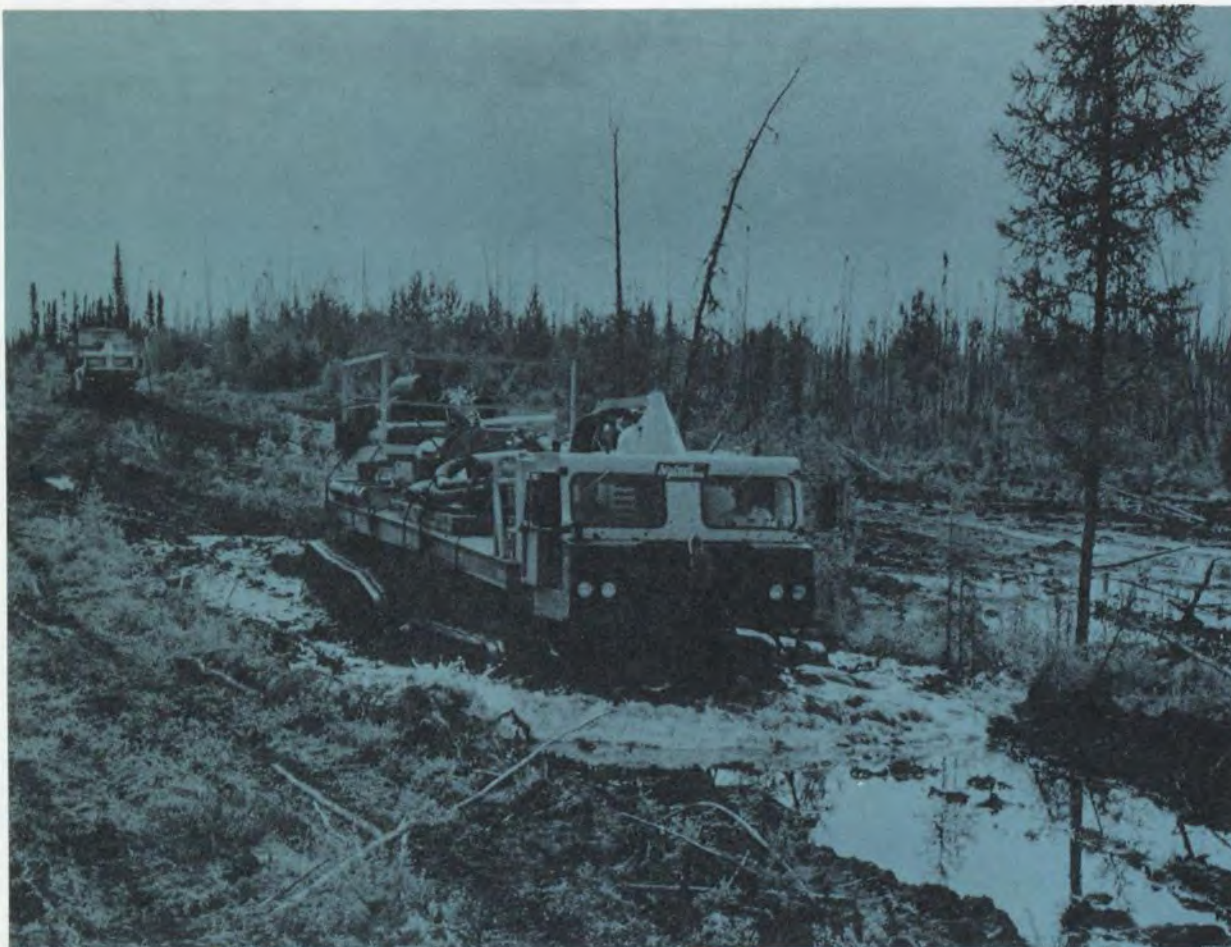
The Nodwell 110, loaded with drilling equipment, has no trouble with a wet, muddy road built through an area of muskeg.
