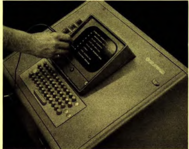
Installed in a teletype unit, a DIVCON monitor shows the main operational directory. The operator is using the light probe to key the passenger service sub-directory.
