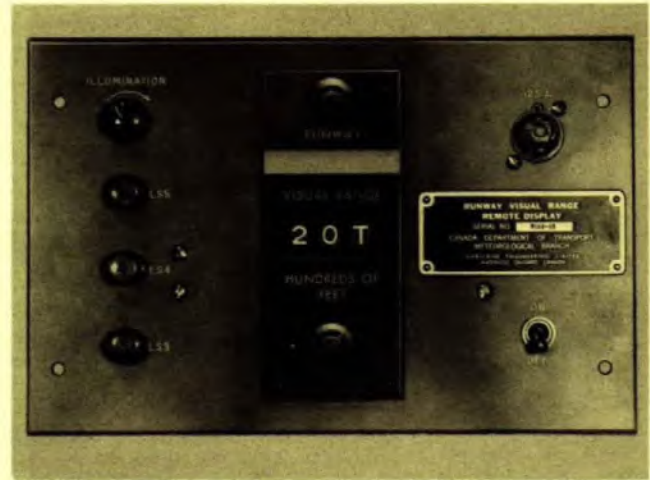
In the front panel of the runway visual range computer, the digits 20-T indicate visibility is 2,000 feet (600 metres) and the unit is under test.
