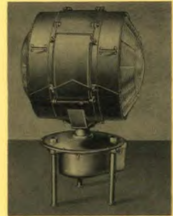
Crouse-Hinds' DCB-36 standard airport rotating beacon has 36-inch (914.4 mm) diameter lenses at each end of the heat-radiating aluminum alloy housing throwing two powerful beams from one standard beacon 1,000-watt lamp.
