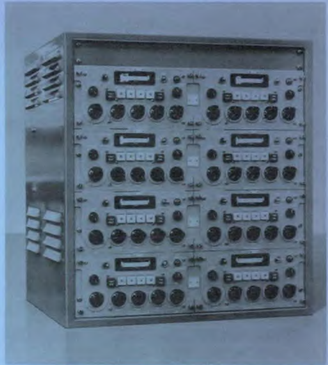
Eight remote control assemblies are shown mounted in one cabinet. Normally they would be installed in an operator's console. This particular assembly is set up for the remotely tuned DDR-506 synthesized MF/HF receiving system used in the Apollo re-entry communications network.
