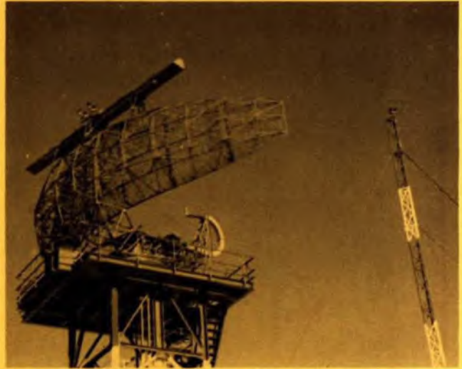
The Raytheon high gain (34 db) antenna has a dual rotary RF joint to allow both primary and secondary radar operation and a choice of circular polarization of RF energy by remote switching.
