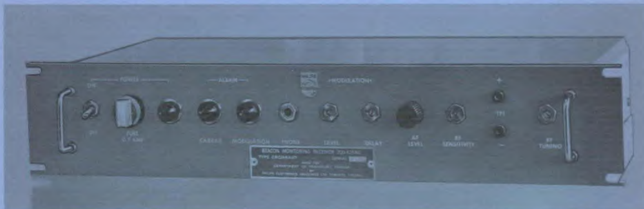
The Philips radio beacon monitoring receiver monitors beacon transmitter output and signals faulty performance.
