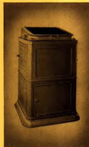
Crouse-Hinds rotating beam ceilometer projector transmits a 1,300-watt modulated light beam at the cloud base every six seconds (left).
