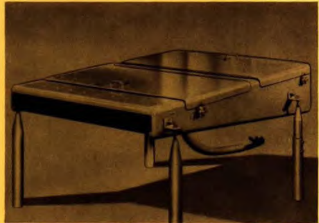
Seen from the front, a VASIS unit showing the rectangular light beam aperture, adjustable legs, and hinged lids for easy maintenance. The four individual lamp cables run to underground insulating transformers.
