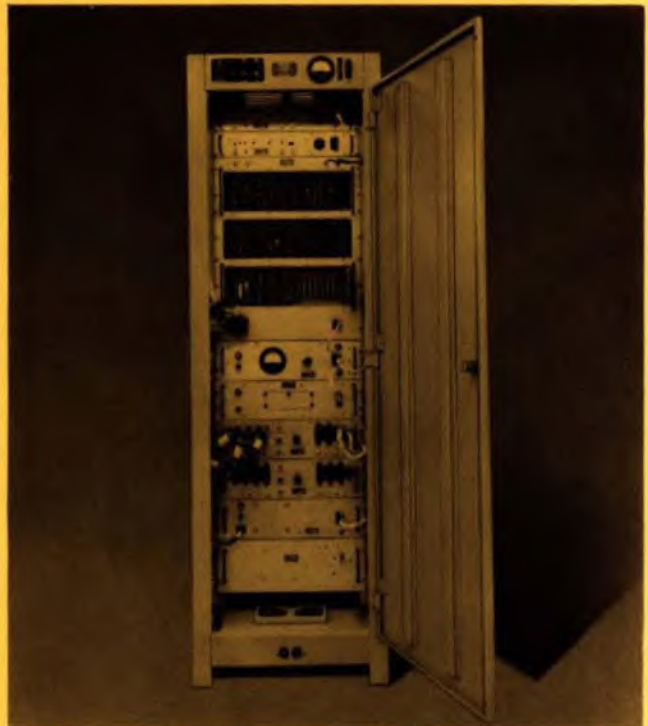
Secondary surveillance radar is an addition to a primary system and is operated in conjunction with it. These units are operating at every major Canadian airport.
