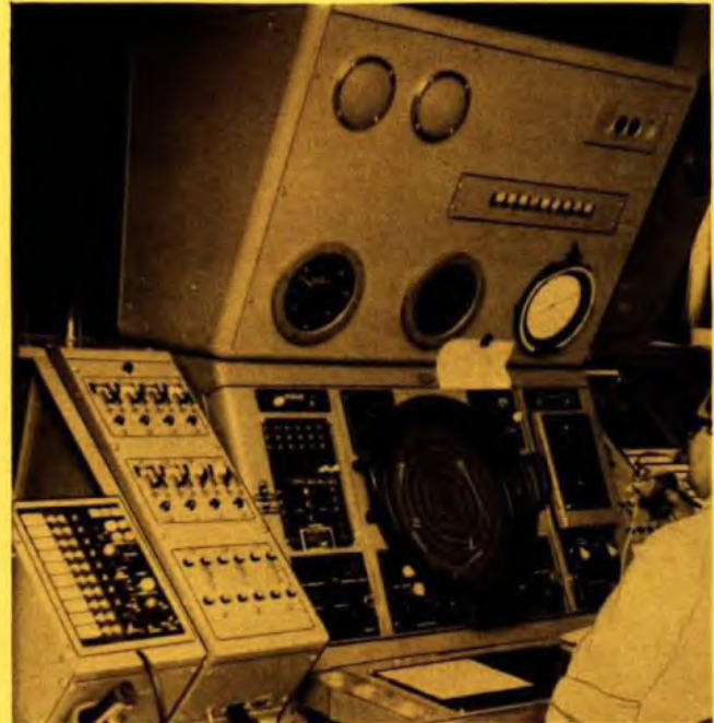
Here is the indicator panel used in Raytheon's AASR. Bright display systems which permit radar signals to be shown on a TV screen are incorporated in latest models.
