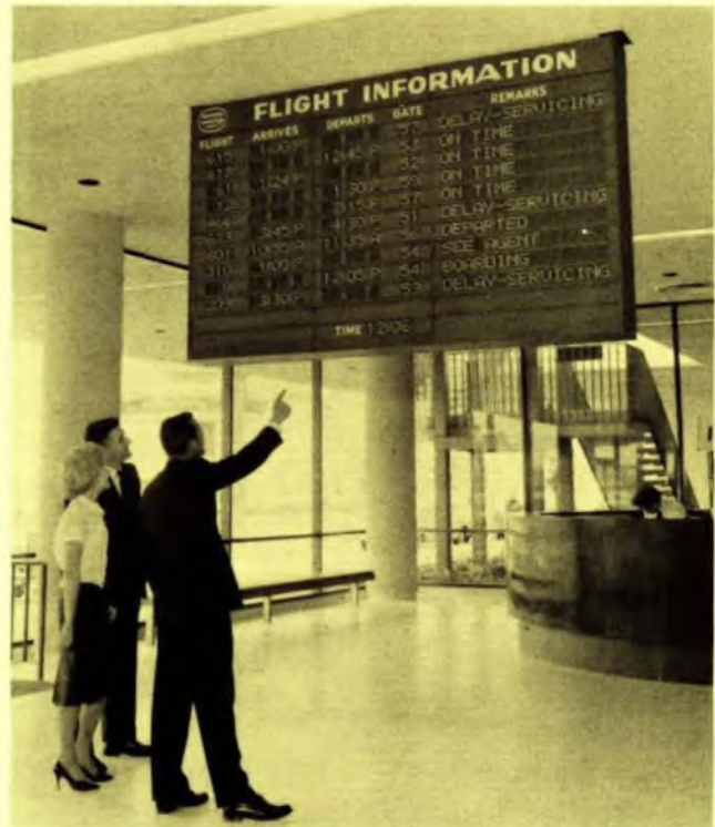
This 300-character Ferranti-Packard flight information board has been in operation at the Western Airlines terminal at Los Angeles, California, since March, 1962.
