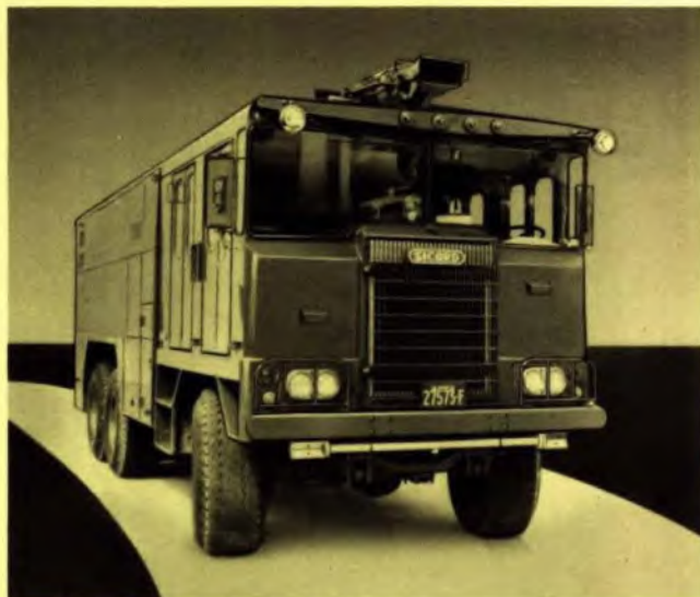
The powerful six wheel drive Pyrene/Sicard fire-fighting and crash rescue vehicle can get to a crash scene quickly over off-the-airport terrain. It can discharge over 800 Imperial gallons (3,600 litres) of fire killing foam.
