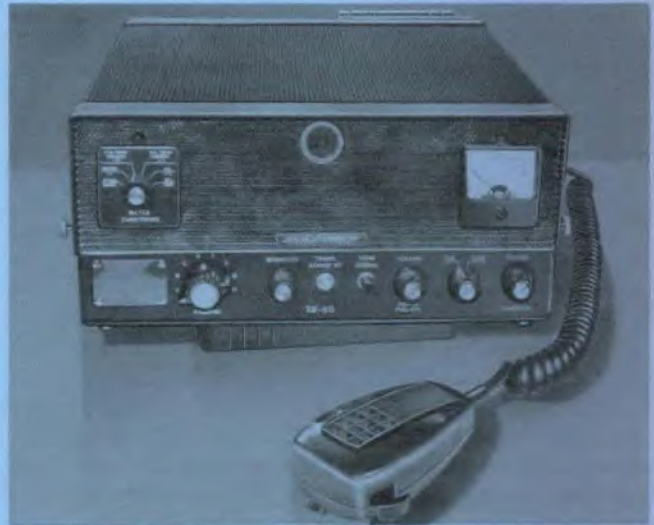
For base, field and airborne operation, the SB-60 weighs only 8 pounds 5 ounces (3.7 Kg), and is simple to operate. It measures only 5 by 9 by 11 inches (127 by 228.6 by 279.4 mm).
