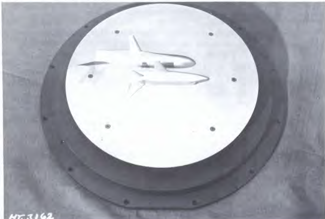
Half Models of Space Shuttle (Booster and Orbiter) Mounted on Reflection Plate of NAE 30-inch Supersonic Wind Tunnel
