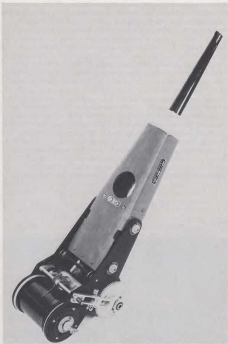
Figure 20 Storable Tubular Extendible Member (STEM) — developed from the antenna units used on Alouette 1.
