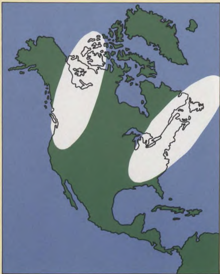
Figure 55 Earth coverage provided by the Hermes antenna beams for one specific experiment when the satellite was at 116° W longitude.
