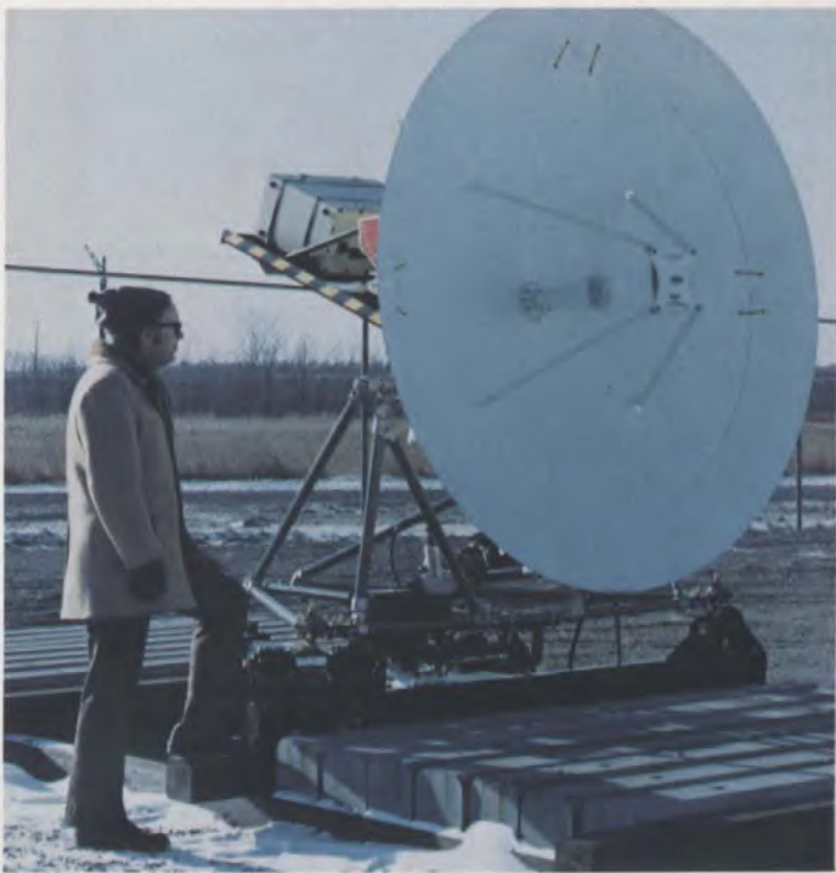
(c) TV interactive terminal (TV-receive, telephony-transmit) with 2 m diameter antenna.
