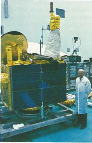
Anik B, the world's first hybrid communications satellite operating in 6/4 GHz and 14/12 GHz bands, is readied for launch at the Kennedy Space Center.
