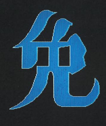
The secret of Telidon is in it's highly efficient coding scheme – The Picture Description Instructions "PDIs" which describe images in terms of basic geometric elements such as points, lines, arcs, rectangles and polygons. Telidon terminals can handle non-Latin characters, ideographic symbols or cursive scripts as well as the widest range of videotex attributes such as color, motion, overlays and display resolution.
