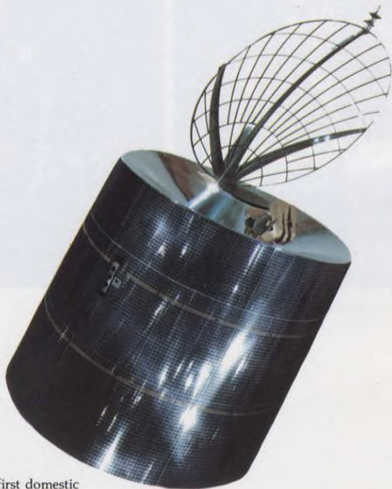
Anik A, world's first domestic communications satellite to be placed in geostationary orbit.
