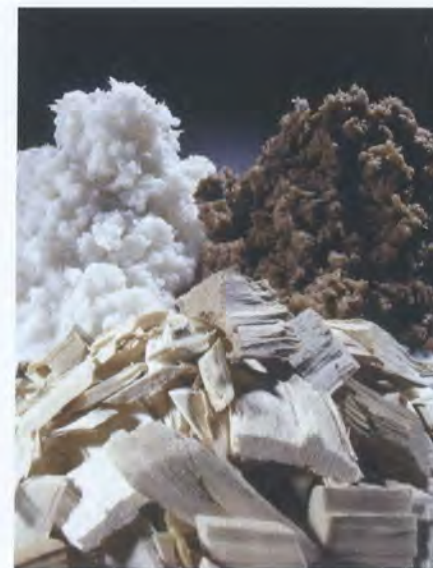
ABOVE: a more environment-friendly and economical way to produce bleached pulp. In 2002, more than 2 million tons of brown pulp produced from wood chips were pretreated using xylanase enzyme before the bleaching process. This led to a decrease in the use of bleaching chemicals and a reduction in harmful chlorinated byproducts.
