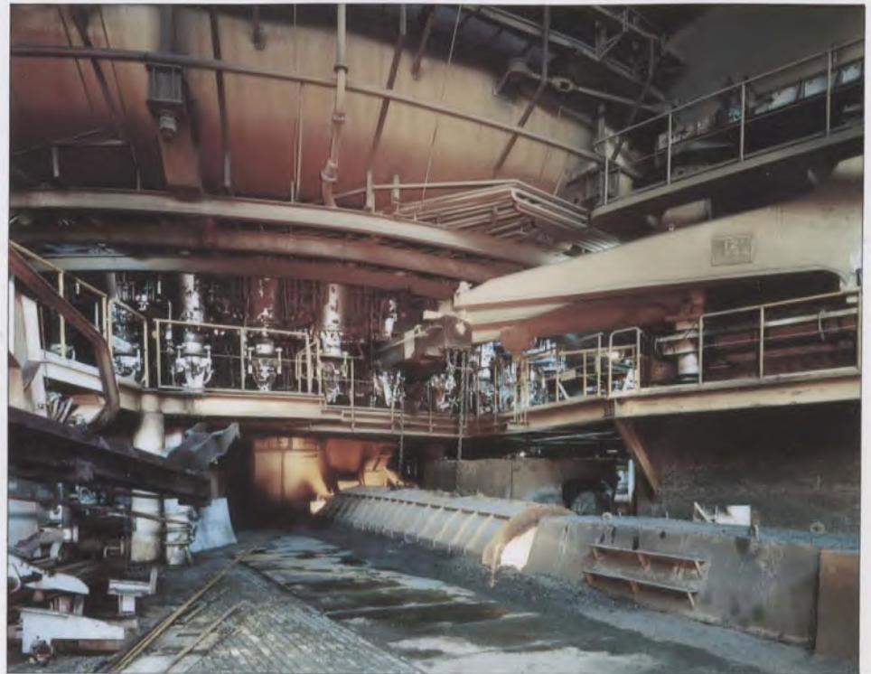
Discharging of hot metal from a blast furnace.
