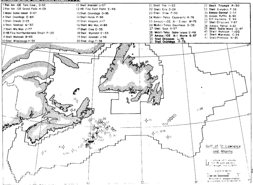
Shell's first Scotian Shelf test, 20 miles southwest of Sable Island, was actually a marginal dry gas discovery at around the 9,000 feet level. Operators have announced that indications of hydro-carbons have been found in several other wells on the Scotian Shelf. On the Grand Banks, a show of gas was recorded while non-commercial oil showings were reported by Amoco in the second well of their current drilling programme.
