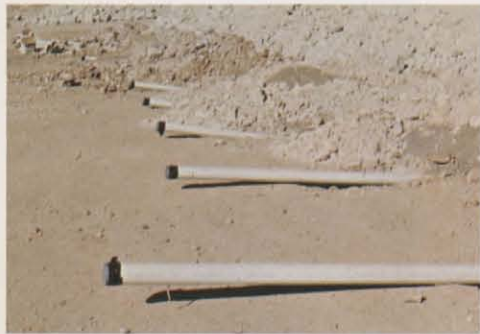
BIOLOGICAL LEACHING OF COPPER — During 1970 large test dumps of copper ore were set up at Cananea, Mexico, and Tyrone, New Mexico, under conditions for accelerated leaching previously determined through laboratory experimentation. The photograph shows aeration pipes extending from the base of one of the 50,000 ton dumps.
