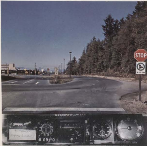
B.C. RESEARCH HIGHWAY SCANNER —The scanner rapidly records a photo-inventory of road conditions on 16mm color film. Each frame of the film records road conditions, including signs and obstructions, together with such data as the vehicle's speed, altitude, and the centrifugal forces acting upon it. One unit, built for N. D. Lea and Associates, is being used to examine the highway system in Tanzania.
