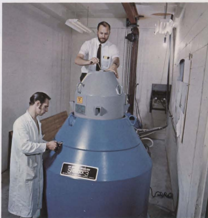
NEUTRON ACTIVATION ANALYSIS — In cooperation with Atomic Energy of Canada Limited, a "Sherlock 3" neutron activation unit has been installed at B.C. Research for studying its application to mineral analysis and to on-stream analysis of ore at its various milling stages. Other applications include "tagging" of wood chips and other material for on-line process analysis, and the production of short-lived isotopes.
