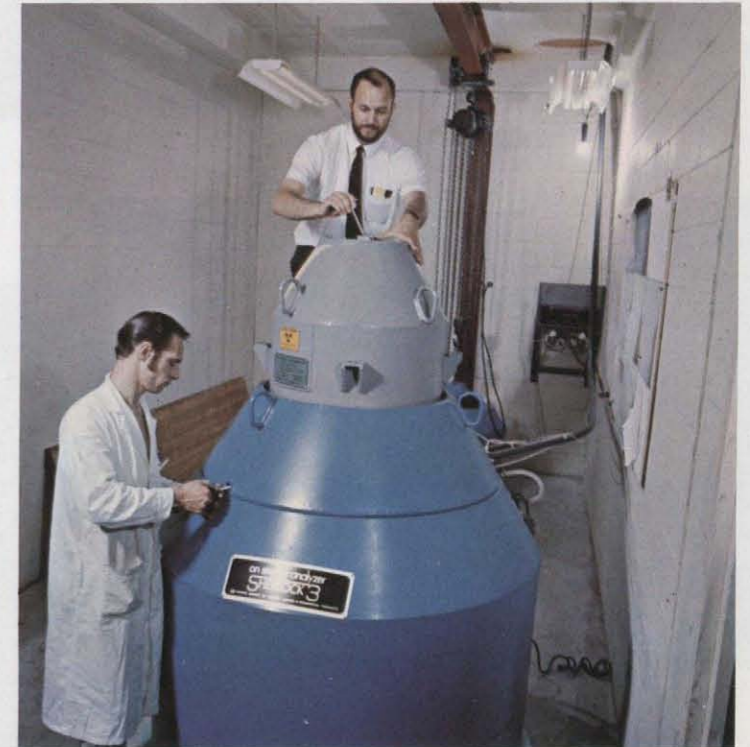
NEUTRON ACTIVATION ANALYSIS — In cooperation with Atomic Energy of Canada Limited, a "Sherlock 3" neutron activation unit has been installed at B.C. Research for studying its application to mineral analysis and to on-stream analysis of ore at its various milling stages. Other applications include "tagging" of wood chips and other material for on-line process analysis, and the production of short-lived isotopes.
