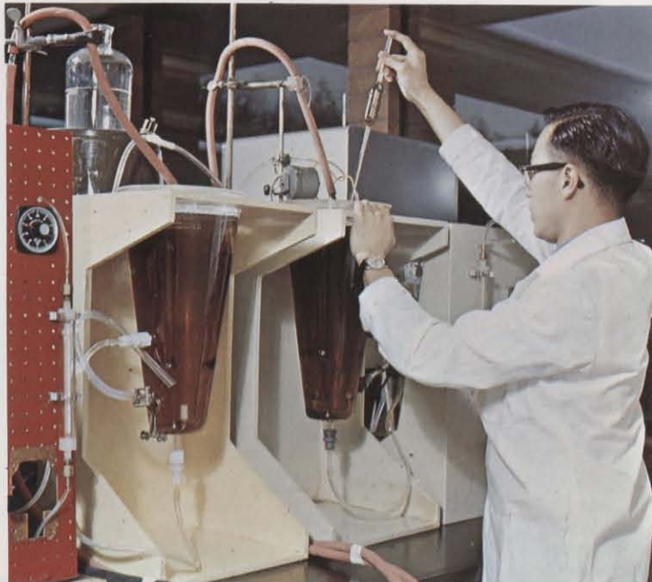
BIOTREATMENT OF INDUSTRIAL WASTE — Operation parameters of the low-rate activated sludge process are studied on bleached kraft mill effluents.
