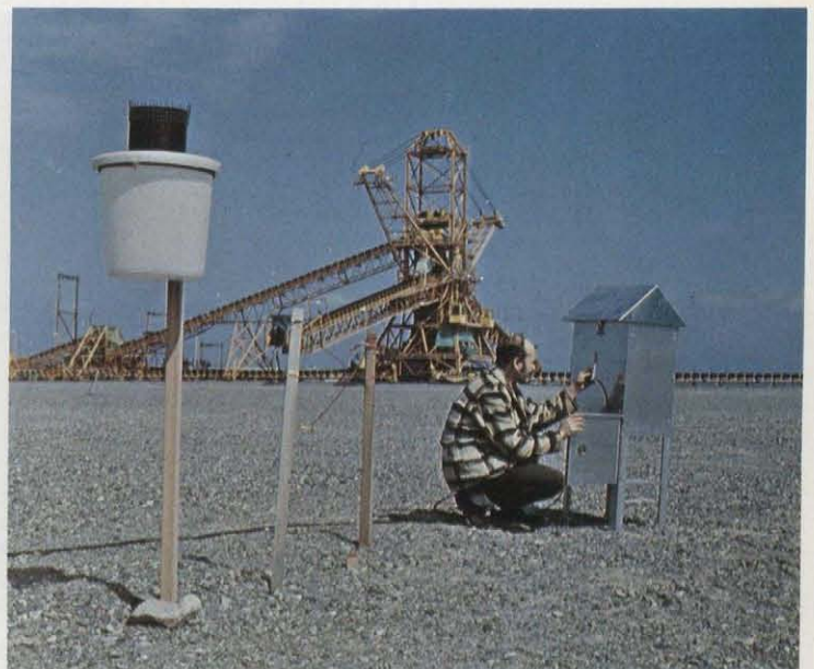
DUSTFALL SURVEYS — B.C. Research measures fallout and suspended particulate matter in many industrial and urban locations. Here monitoring is carried out at the Roberts Bank Superport.
