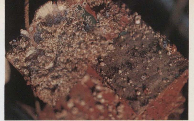
BARNACLE CONTROL — Barnacles grow luxuriantly in B.C. waters causing fouling of boats and marine structures. An anti-barnacle coating (right quadrant) shows promising effects.
