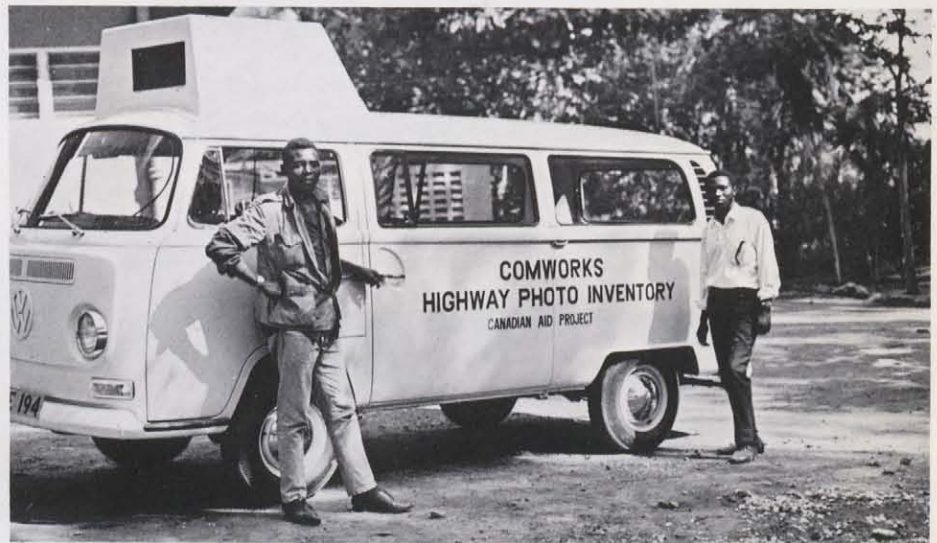
B.C. RESEARCH HIGHWAY SCANNER —The scanner rapidly records a photo-inventory of road conditions on 16mm color film. Each frame of the film records road conditions, including signs and obstructions, together with such data as the vehicle's speed, altitude, and the centrifugal forces acting upon it. One unit, built for N. D. Lea and Associates, is being used to examine the highway system in Tanzania.
