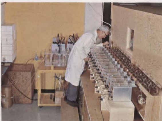
ODOR THRESHOLD MEASUREMENT — This apparatus supplies accurately controlled and graded quantities of an odoriferous material for determining the point at which it is just detectable by the human nose. The method used in food technology and in air pollution studies.
