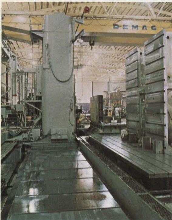
ALIGNMENT SERVICES — The machine ways of this Shibaura Boring Mill are regularly checked by our optical engineering group for S. Madill Ltd.
