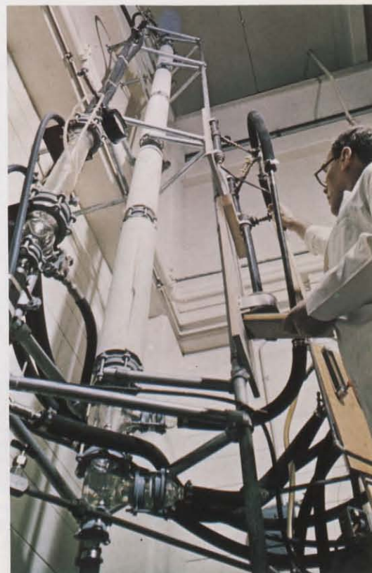
PROCESS DEVELOPMENT —One of our chemical engineers checks a steam stripping system in an attempt to reduce oil refinery waste-water pollution.
