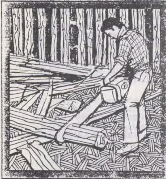
Slashing a log with a chainsaw. Make a notch on the side of the log. Much easier to cut through the log with a chainsaw. The notch is cut from any angle.
