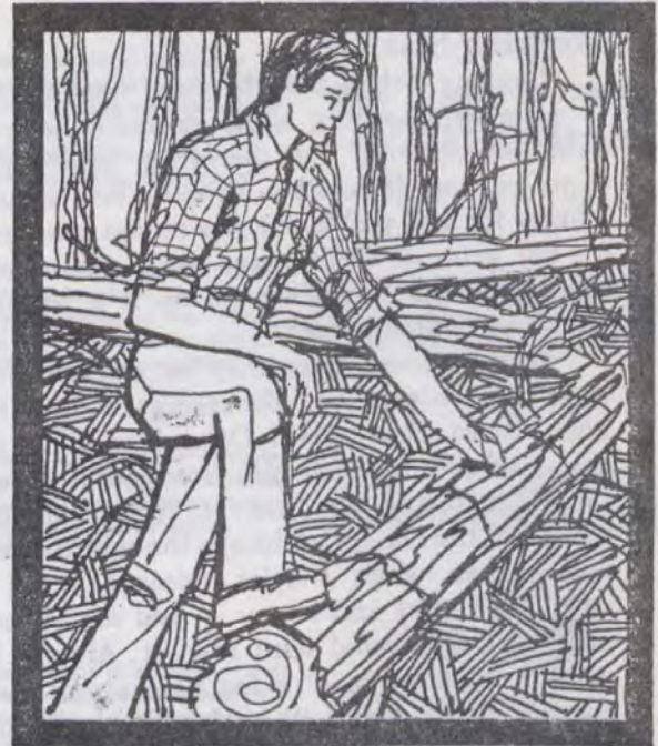
Keep your saw out of the dirt by making a series of partial cuts through a log. Then roll it over and finish the cuts from the other side of the log.
