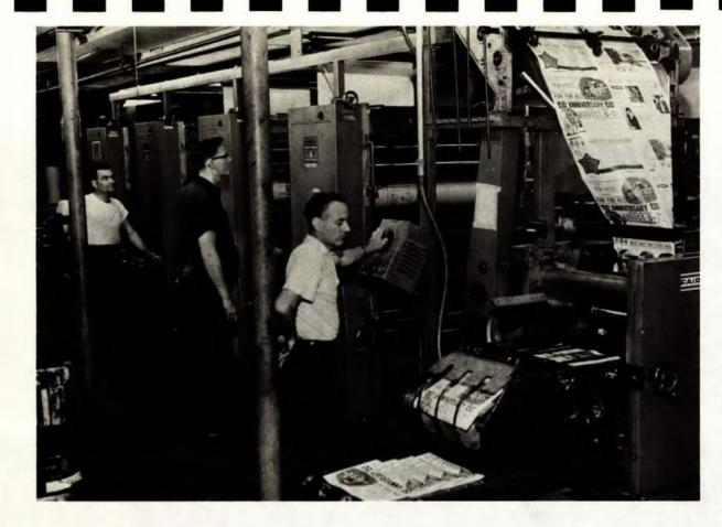
Development grants enabled Kentville Publishing Co. Ltd. to expand this web offset press from two units to four units with the capability of printing in full colour.
