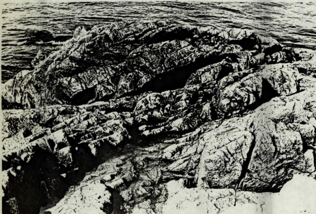
PHOTO NO. 13 Close-up view of the exposed rock showing thin layers and fractures. This type of rock would not easily yield large blocks suitable for armour stone by blasting.
