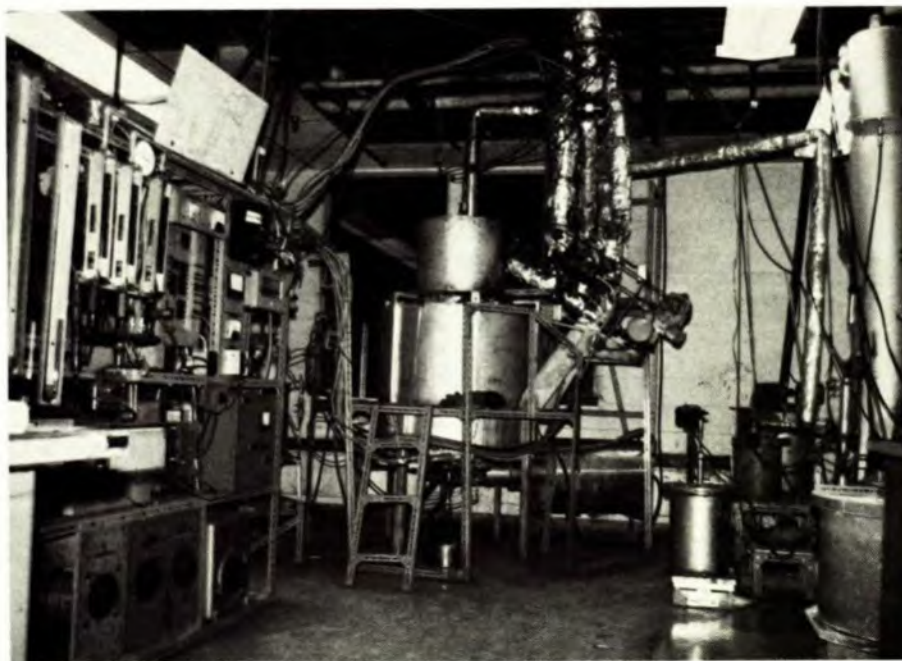
14" Diameter Pilot Fluidized Bed Reactor And Ancillary Equipment
