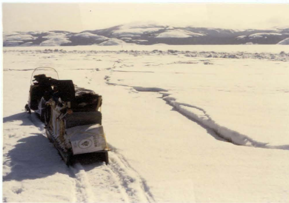
Figure 8b. Example of the track left by the icebreaker SIR JOHN FRANKLIN on its exit leg of the Lake Melville voyage, March 24, 1982. Note the size and extent of the cracking of ice away from the ship's track.
