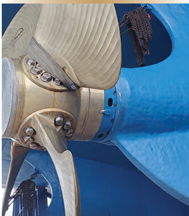
Figure 3. The fixed-pitch propellers fitted on the AOPV are ice-strengthened to meet Polar Class 5 requirements.
