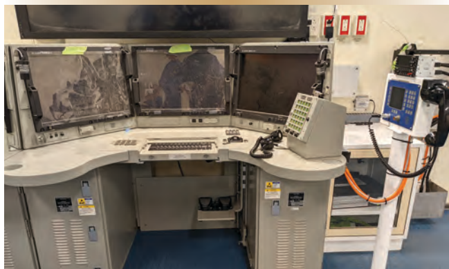
Figure 1. A multi-function console (MFC) for the AOPV combat management system.
