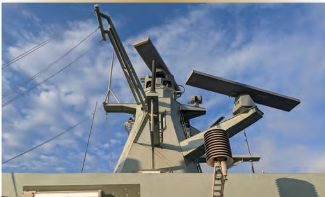
Figure 4. Starboard view of an Arctic and offshore patrol vessel's mainmast, with the surveillance radar on top, and the S-band navigational radar situated lower and forward.
