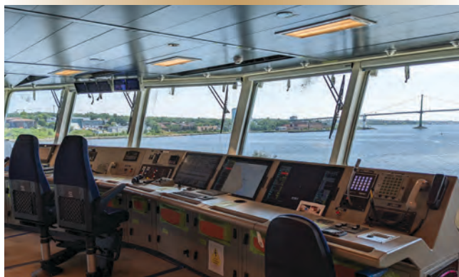
Figure 2. The Integrated Bridge and Navigation System integrates and feeds data to multiple AOPV systems and displays.
