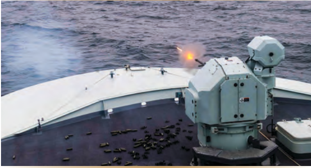
Figure 3. The BAE Mk 38 25-mm Mod 3A machine gun.
