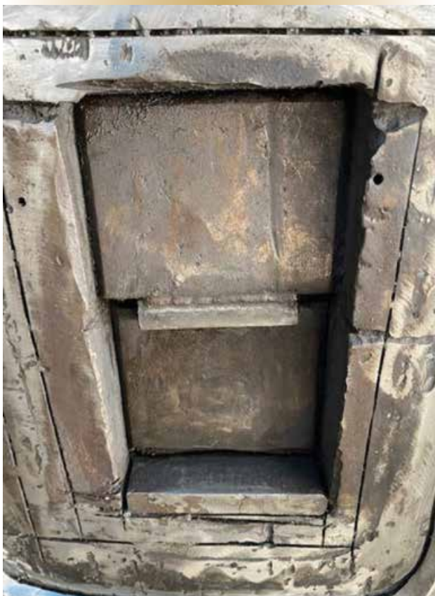
Figure 7. Ville de Québec 's rudder keyway window – May 19, 2022.
