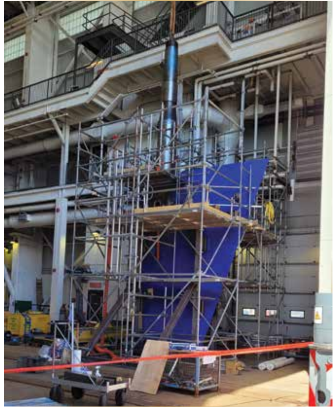
Figure 5. Charlottetown's rudder upright in the jig.
