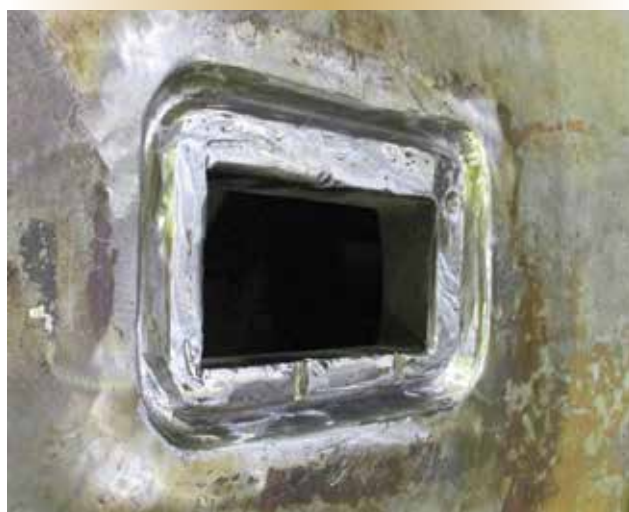
Figure 3. Port keyway with defects excavated (April 27, 2022).
