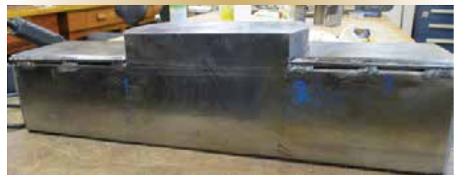
Figure 9. Charlottetown rudder lower securing wedge with shims installed.
