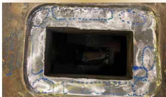
Figure 4b. Port keyway– UT defects (May 6, 2022).
