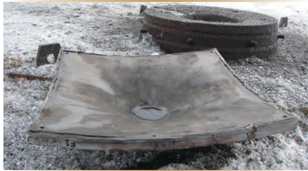
Figure 5. The blast result: A “wash-basin-like” bulged test panel.
