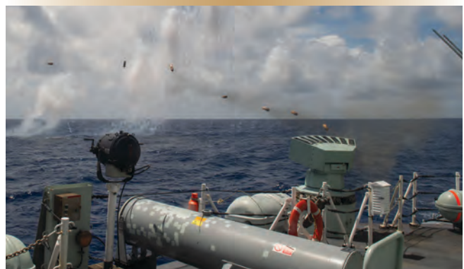
The MASS launcher being loaded with SOPD passive RF decoys... and firing.
