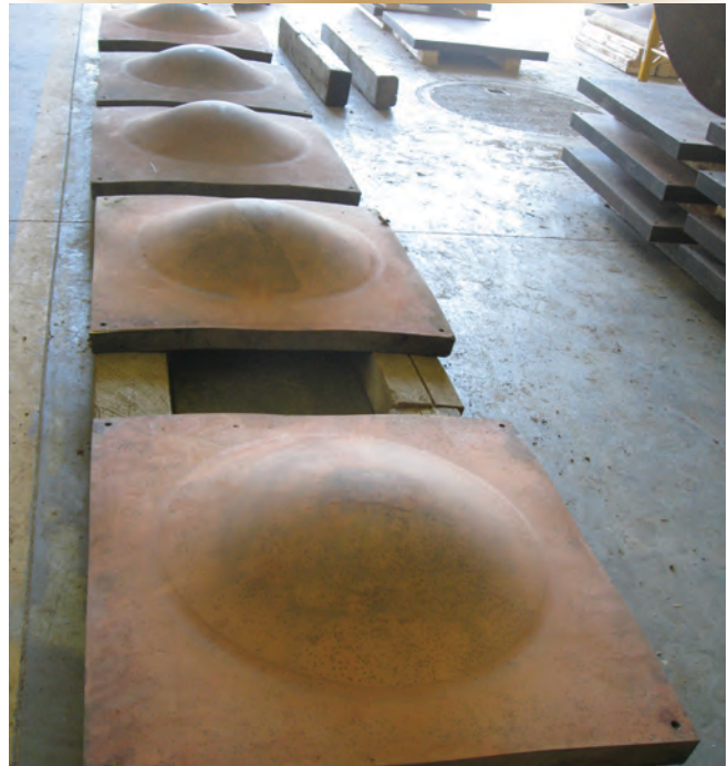
Figure 2. The explosive energy imparted through bulge testing deforms the submarine pressure-hull test panels in a controlled, reproduceable manner.
