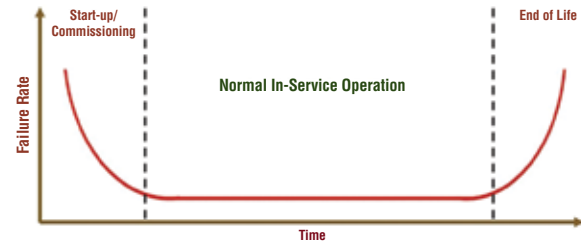
Figure 1. The standard balanced bathtub curve.
