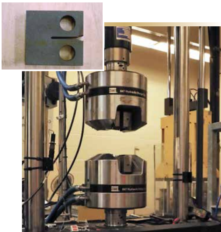
Figure 2. Compact tension specimen with specialized clevis grips and strain gauge, and the hydraulic loading instrument required for fracture toughness testing. Inset: Compact tension specimen.
