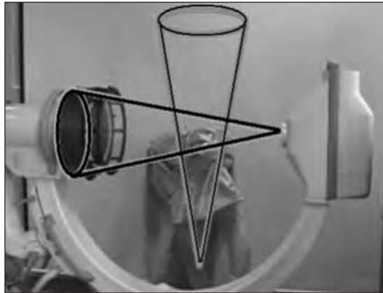
Figure 4.4: Fluoroscopic navigation: Approximates 3D with multiple 2D images.
