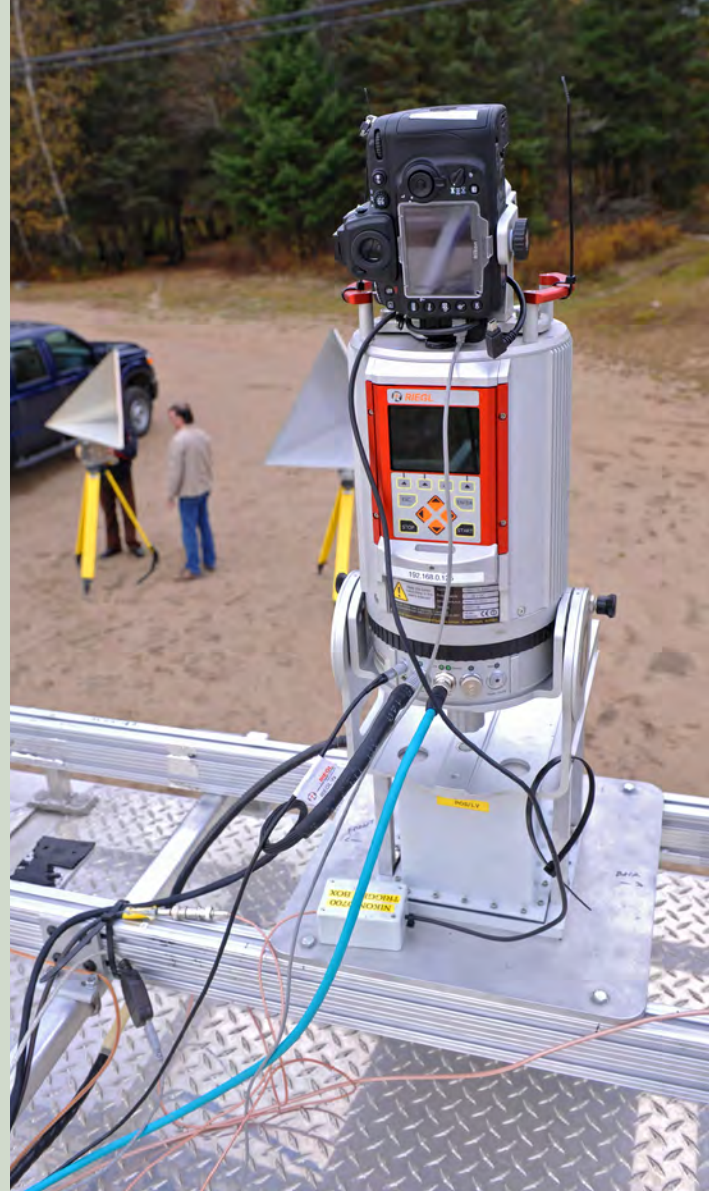
LiDAR system mounted on vehicle for testing at DRDC Valcartier.
