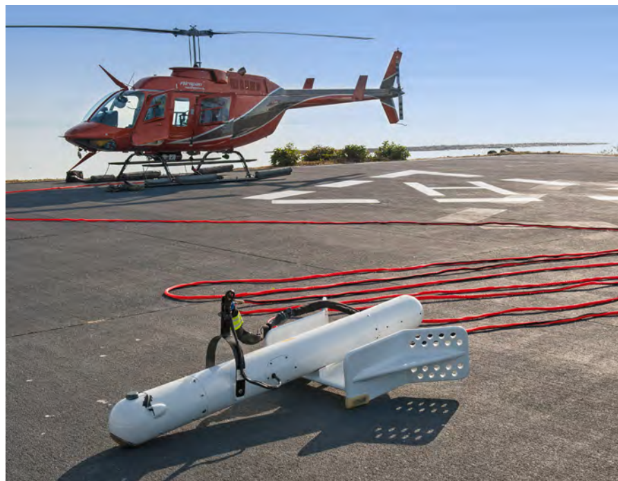
A magnetic anomaly detection trial at the Canadian Forces Maritime Experimental Test Ranges in British Columbia.
