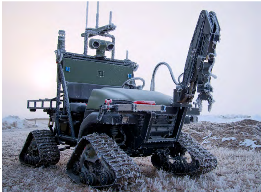
An uncrewed ground vehicle was used to collect samples from radiological threats detected using uncrewed aerial vehicles, during the Radiological Dispersal Trial at DRDC Suffield.
