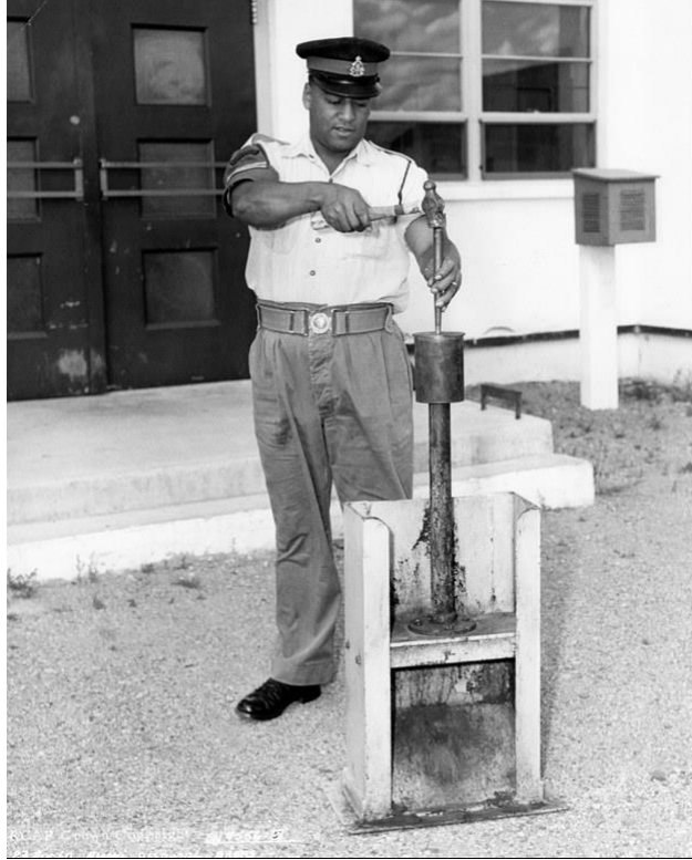
12 - Cpl Lou Brown firing primer in a 105mm cartridge case in 1960. Safety standards have come a long way. Photo credit: CFAD Historical records
