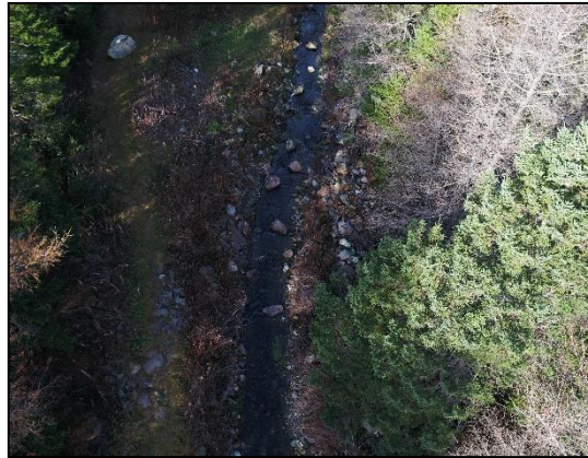
Figure 27. Aerial view of strategic boulder placement at Rocky Pond outlet in Bay Roberts
