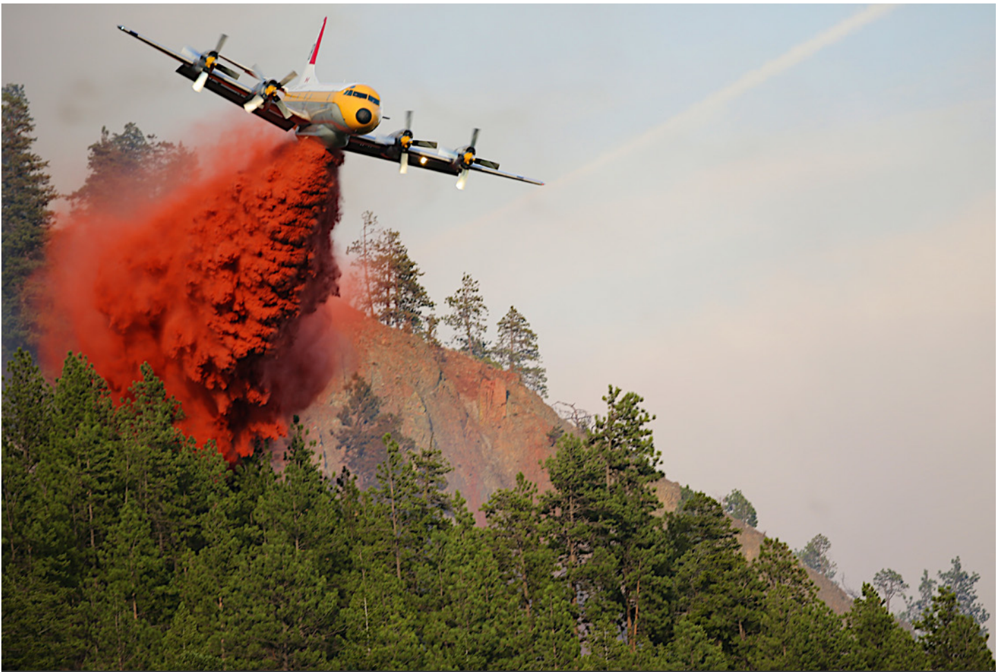
An air tanker drops fire retardant to prevent wildfire spread. Photo by NowMedia.
