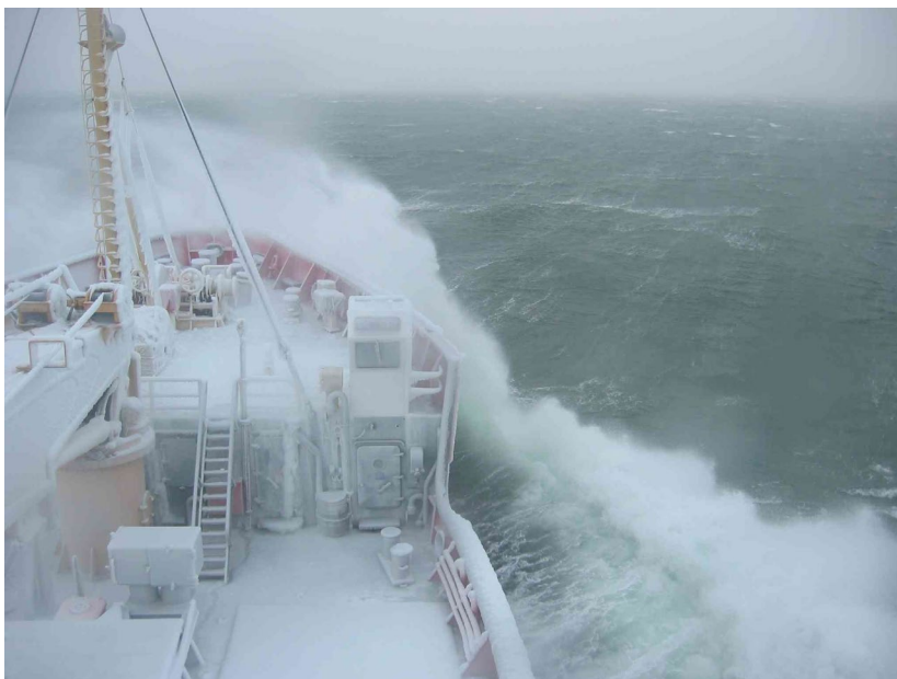
Figure 43 - Severe icing conditions (CCG)
