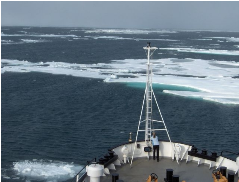
Figure 66 - Vessel encountering strips of multi-year ice (CCG)
