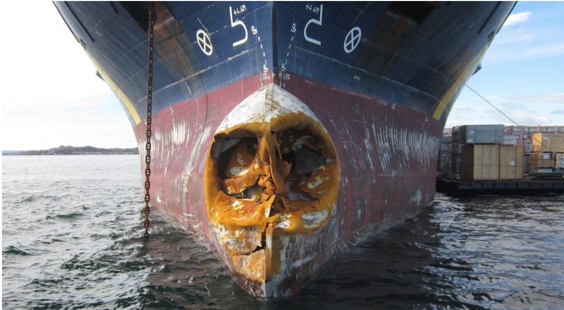
Figure 42 - Bulbous bow of M/V Zélada Desgagnés damaged by ice in Frobisher Bay July 2012 9
