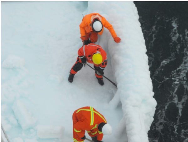
Figure 44 - Crew removing ice from bulwarks
