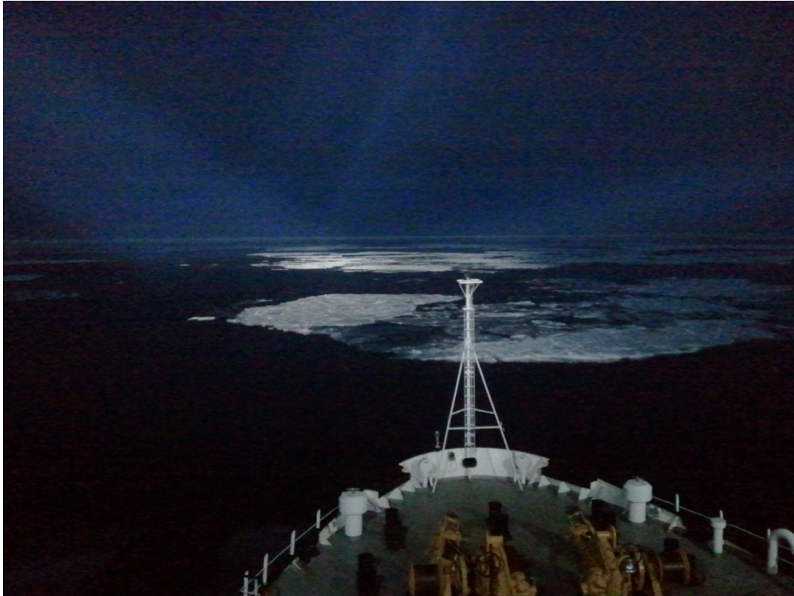
Figure 60 - The use of searchlights when transiting ice at night is essential (CCG)
