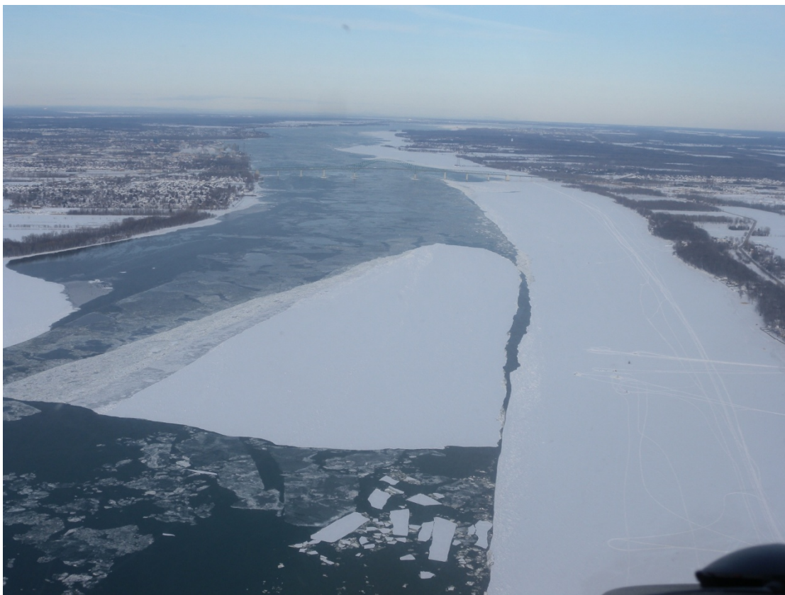
Figure 28 - The vessel channel can be easily blocked if ice is dislodged from the banks (Photo courtesy of CIS)
