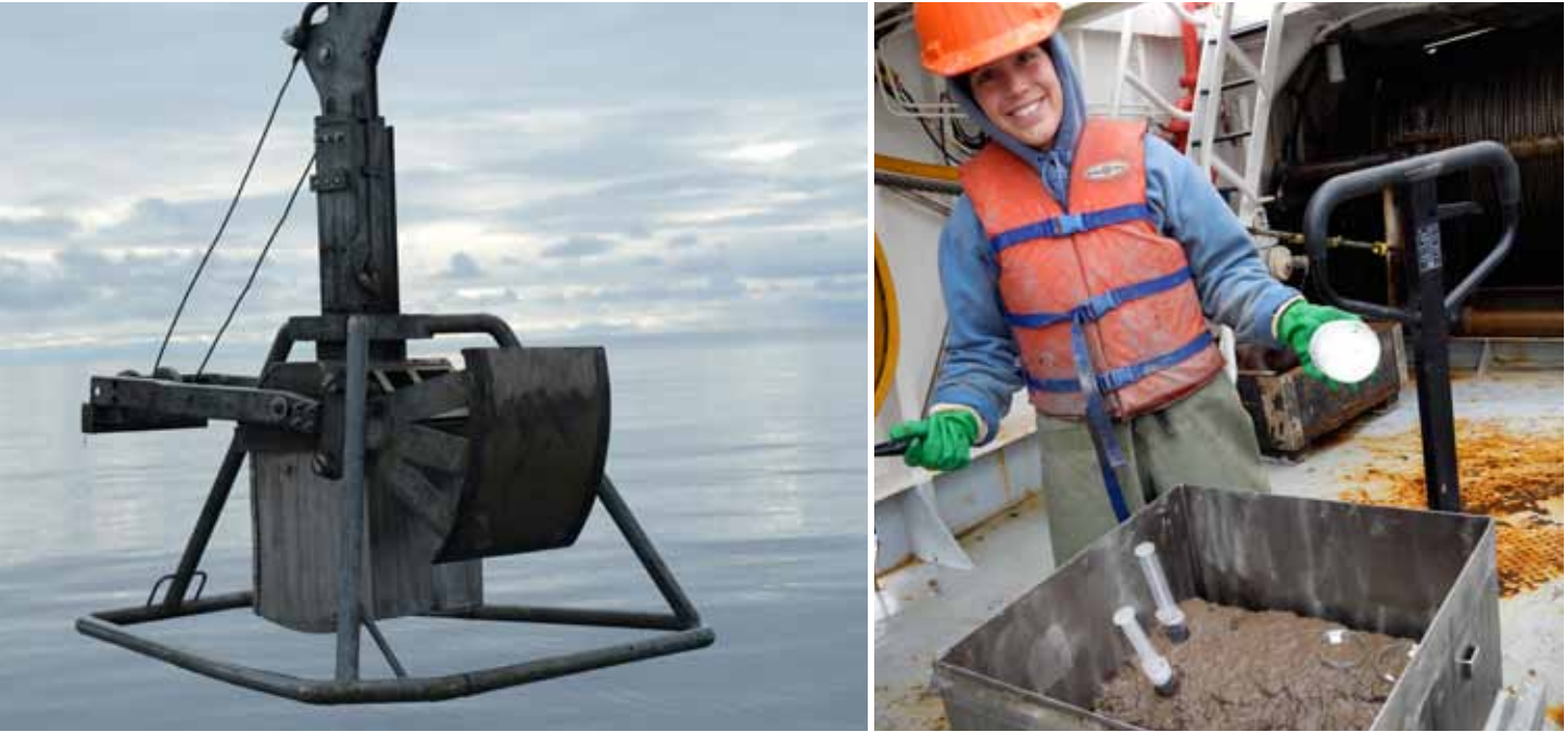
The box corer being deployed from the F/V Frosti (left, Photo by S. Atchison), and Ashley Stasko taking samples from the surface of a sediment core (right, photo by T. Loewen).
